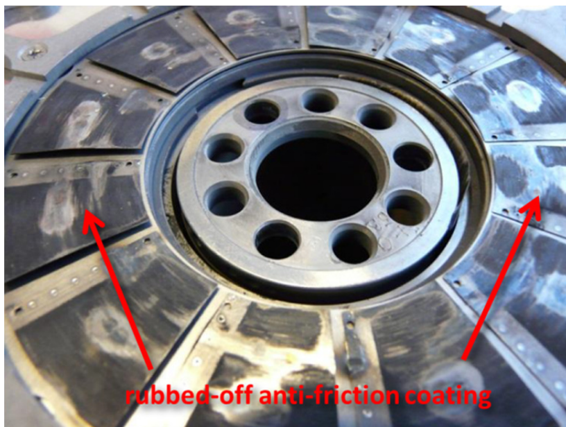
(4) Thrust bearing (anti-friction coating)
