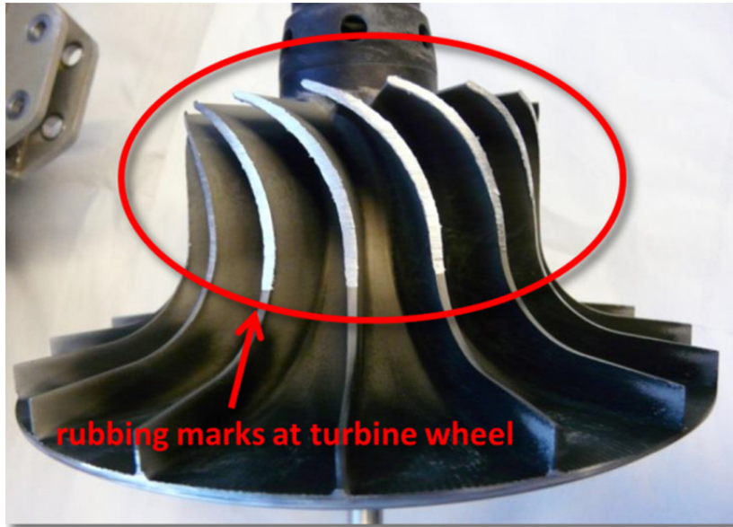
(3) Turbine wheel within the air cycle machine
