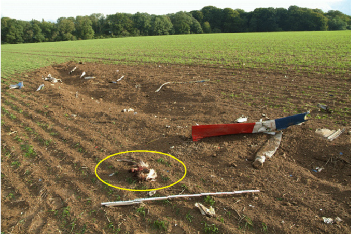
Accident site, view to the south-east, bird cadaver, left aileron and propeller blade
