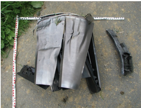
Parts of the nozzle (left); carbon composite structure of the Eurofighter
