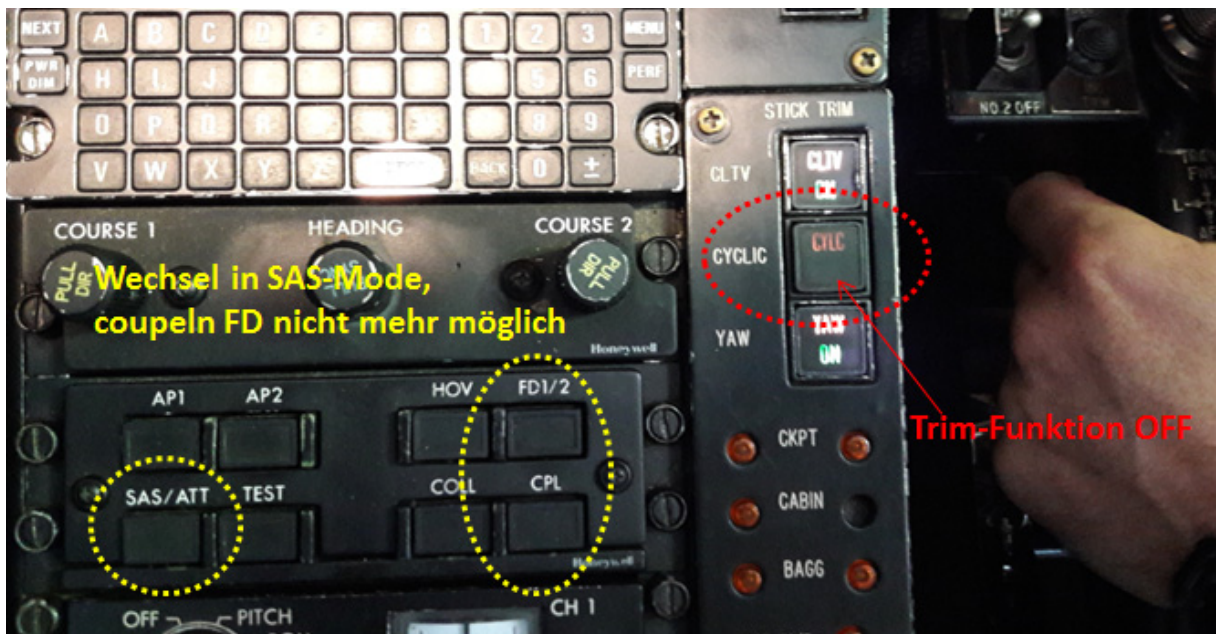
Overview AP and FD panels and the trim push switch
