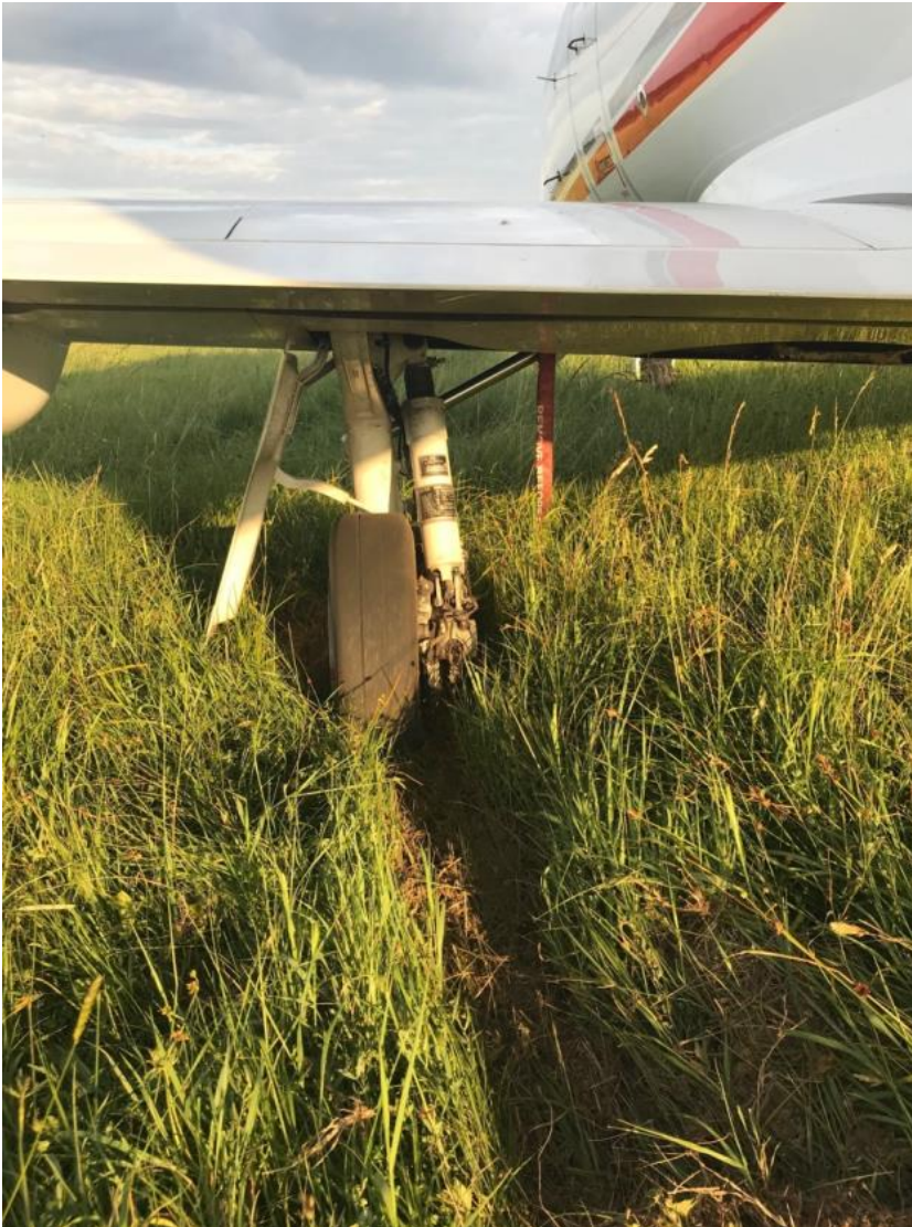
Fig. 3: Left main landing gear with minor damage
