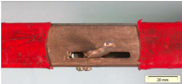
Guidance of the operating lever in the safety bar
