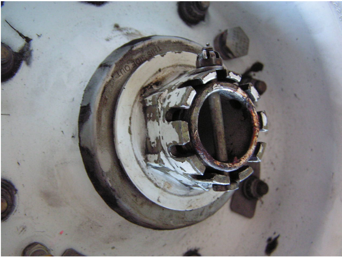
Image 2: Axle with crown nut and safety bolt
