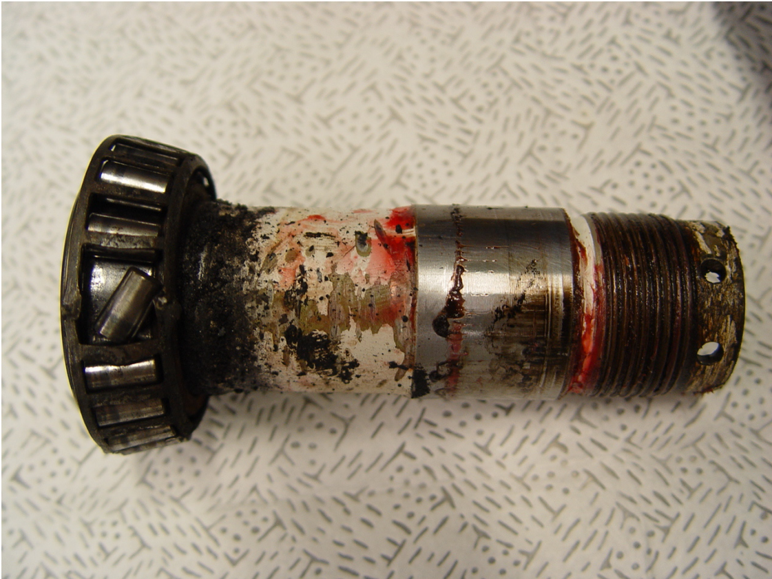
Image 3: Axle stump with destroyed tapered roller bearing
