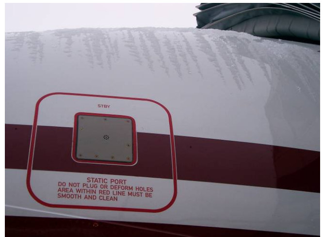
After the landing in Frankfurt, ice was still visible on the aircraft nose over the Static Ports and Pitot Probes.
