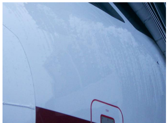
Snow and residual ice on the aircraft nose below the cockpit windscreen after the landing in Frankfurt.
