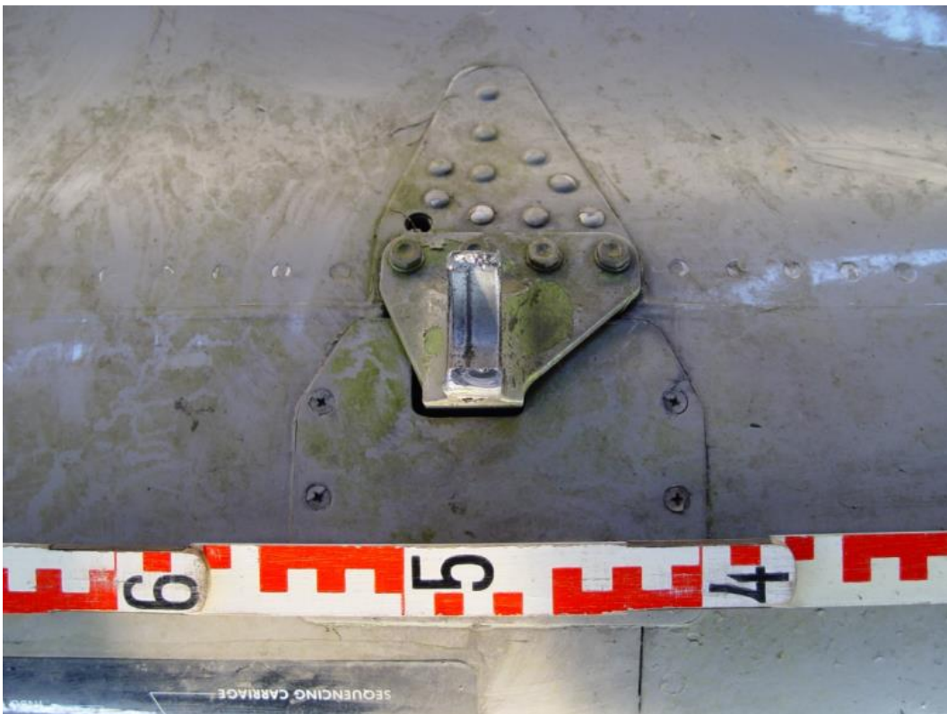
Image 8: Fractured flap attach fitting (bearing seat)
