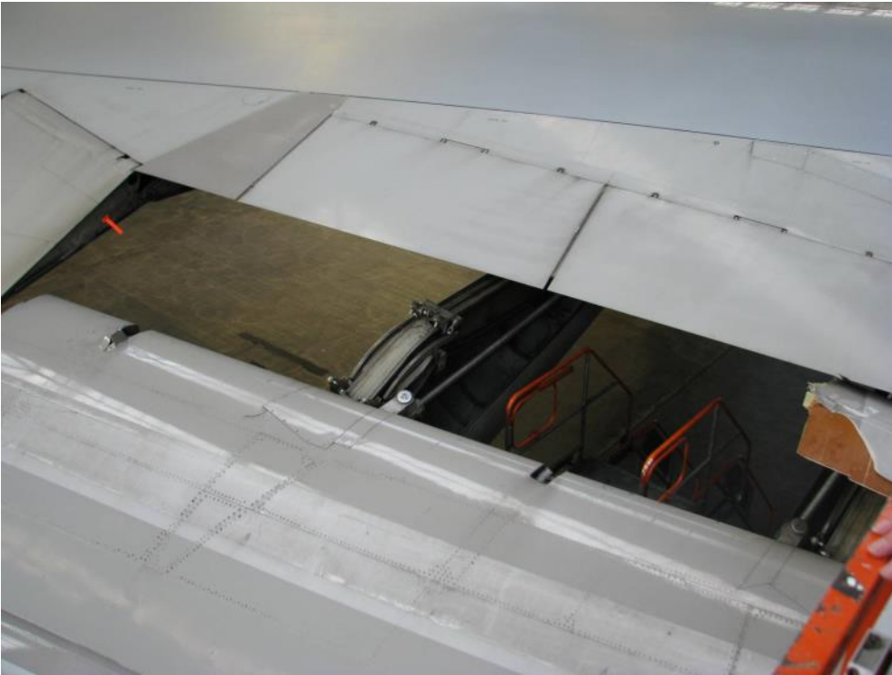
Image 1: Area of the left wing, where the flap part is missing.
