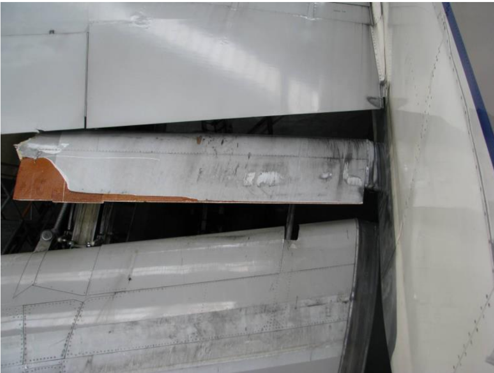
Image 2: Jammed part of the remaining flap
