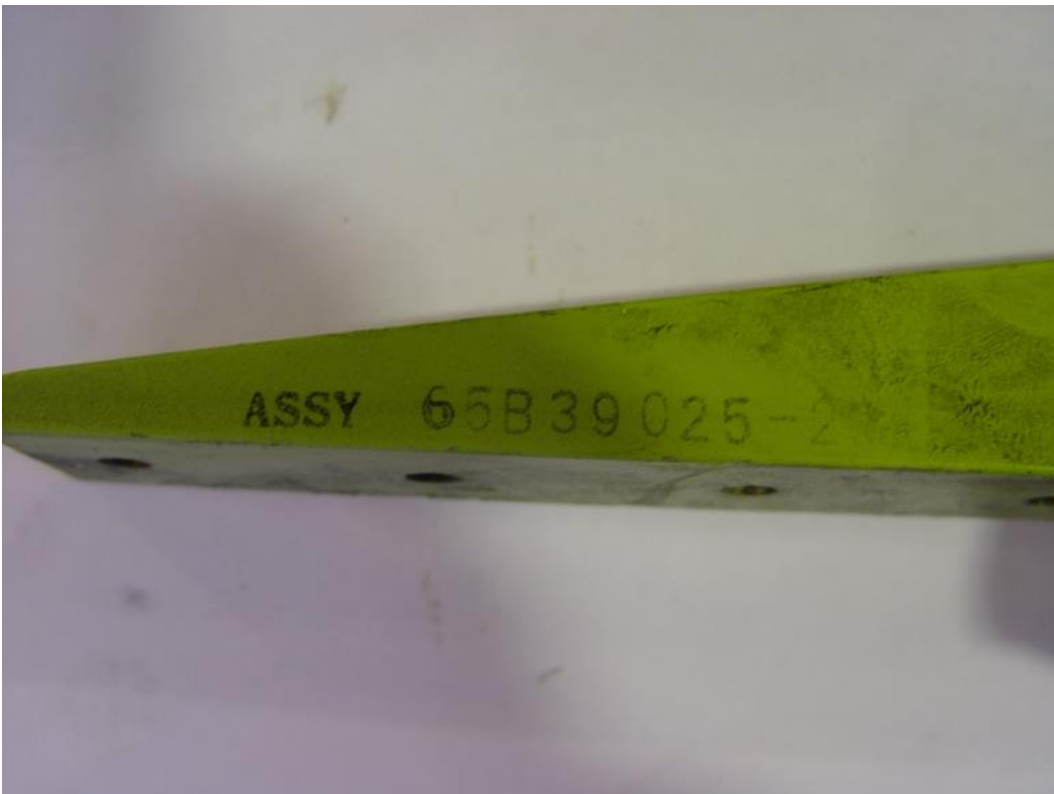
Image 10: Part number of the fractured flap attach fitting
