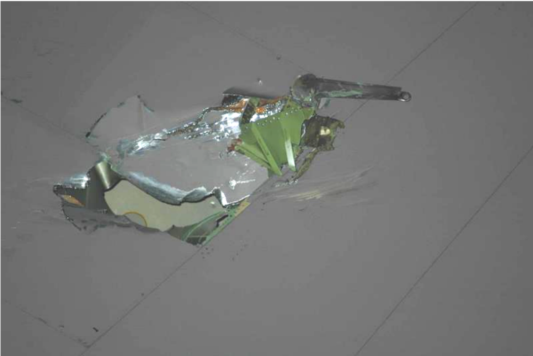
Image 5: Damage on the vertical tail
