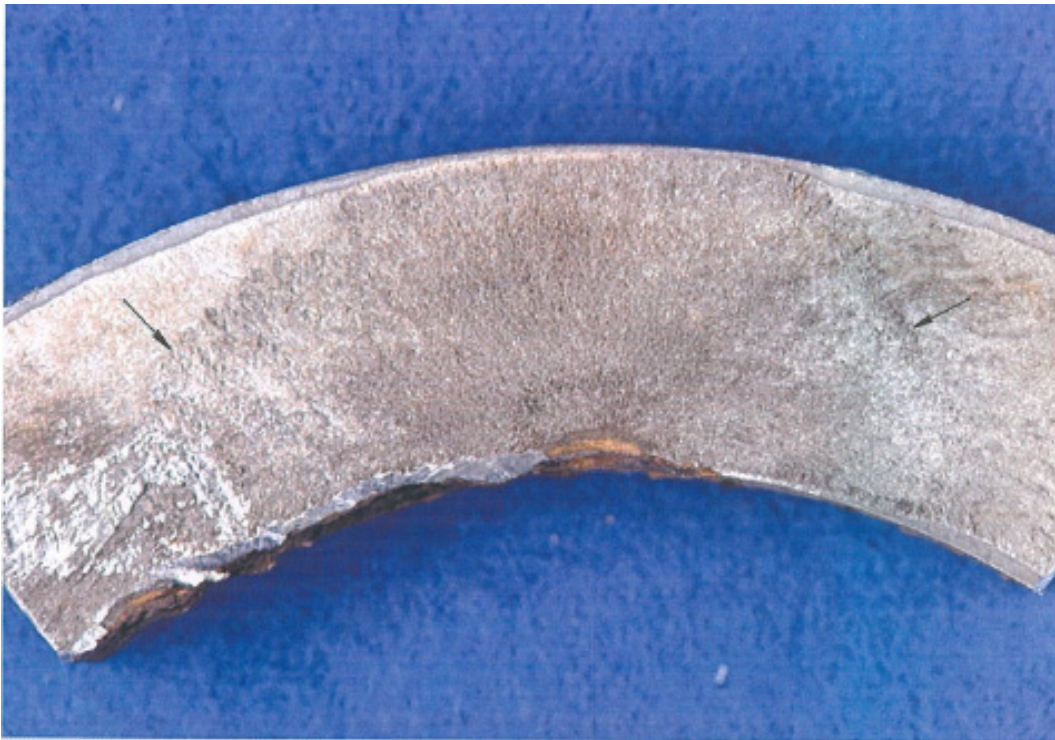
Appendix 9: Thumbnail initial crack (arrows)
