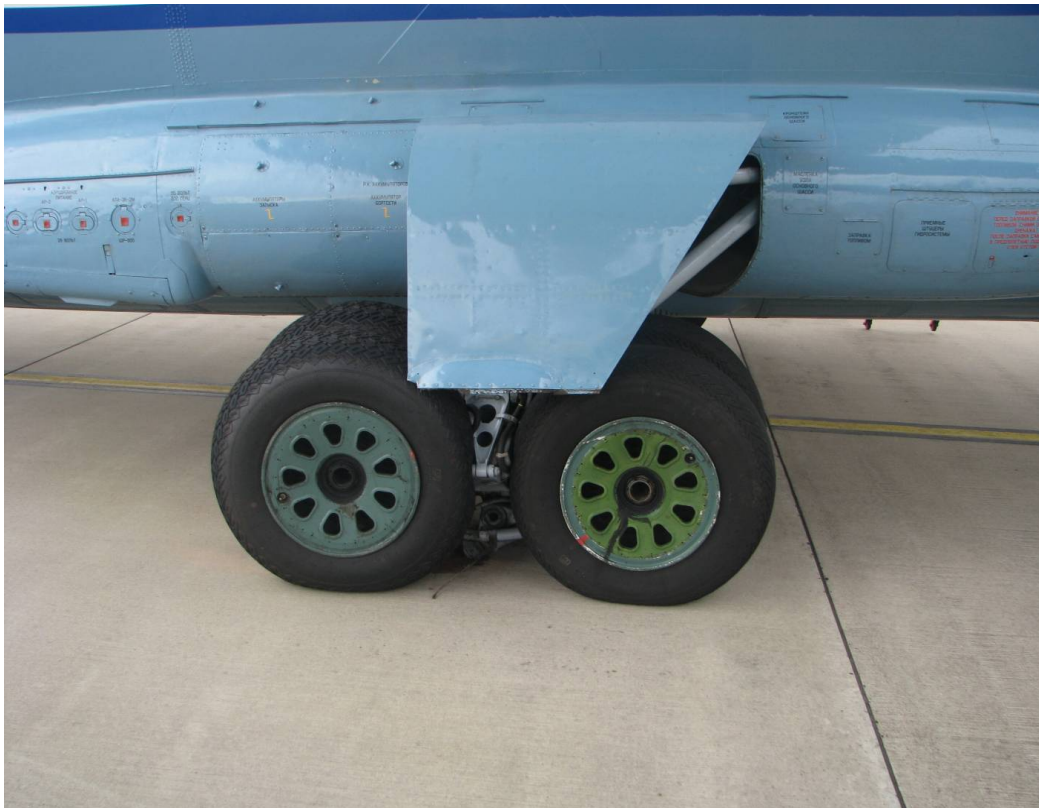
Appendix 2: Damaged right main landing gear
