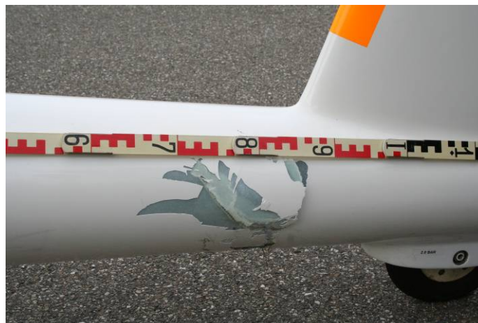
Damage to rear fuselage, DG 300
