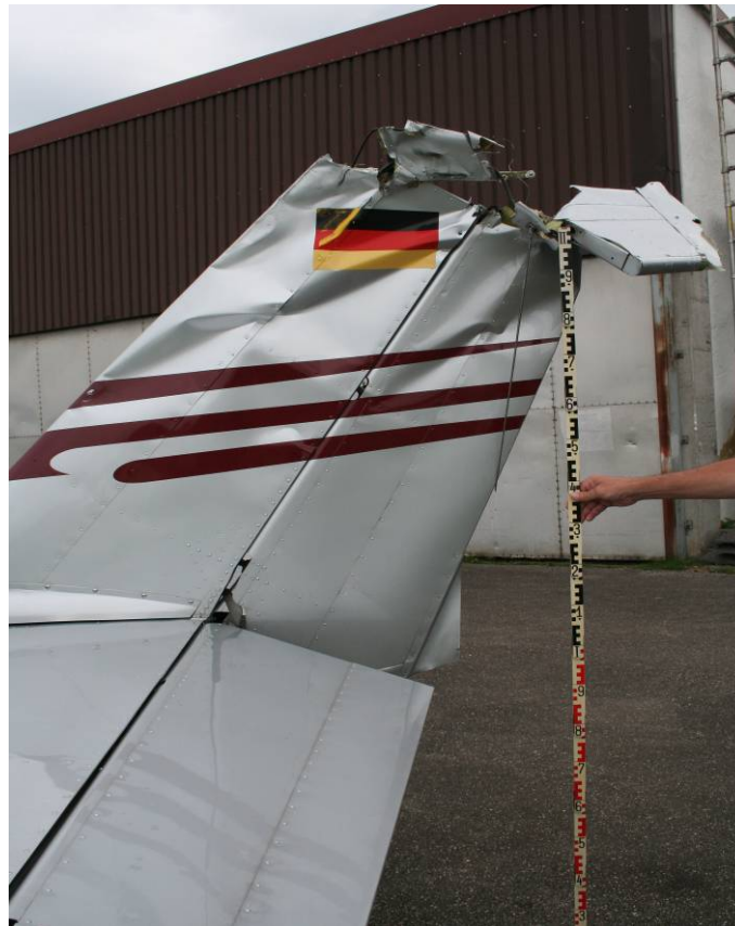
Damage to fin and rudder
