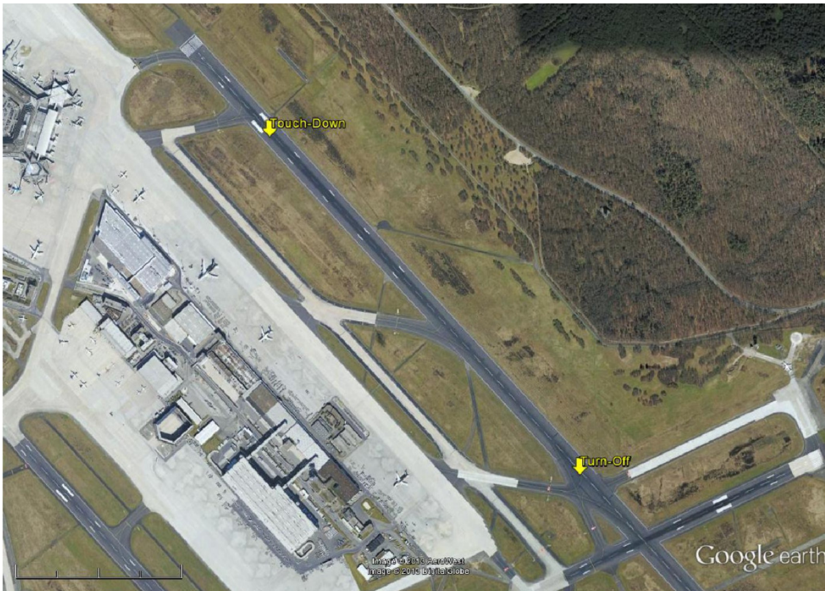
Image 2: Touch-down and turn-off point of the airplane based on the QAR data
