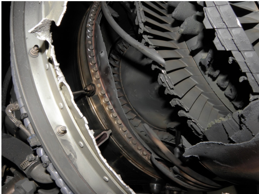
Damaged engine cowling and turbine
