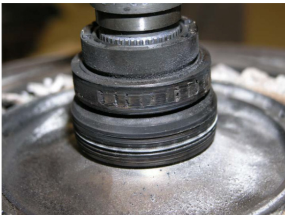
Damages on the rear main bearing and the power turbine
