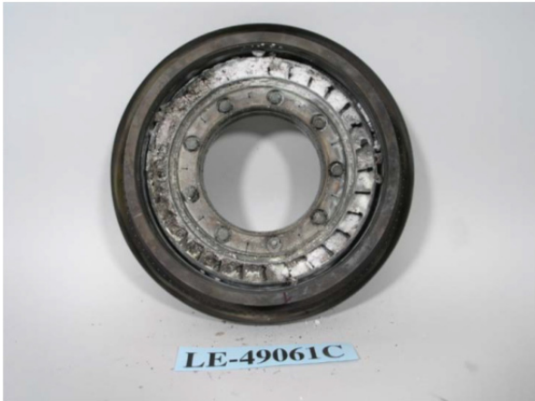
Damage to the nozzle vanes and separated turbine blades
