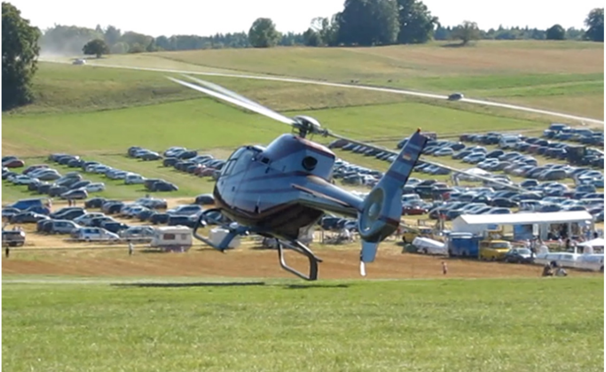
Single image of the accident, the right landing skid "hooks" into the meadow
