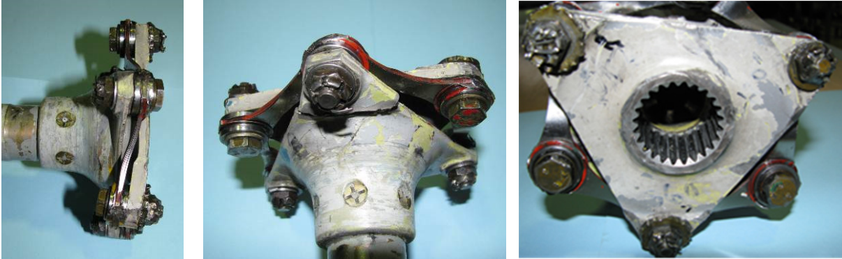
Damages on the rear coupling
