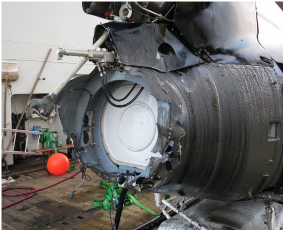
Damages on the aft fuselage section and the Star Flex rotor head
