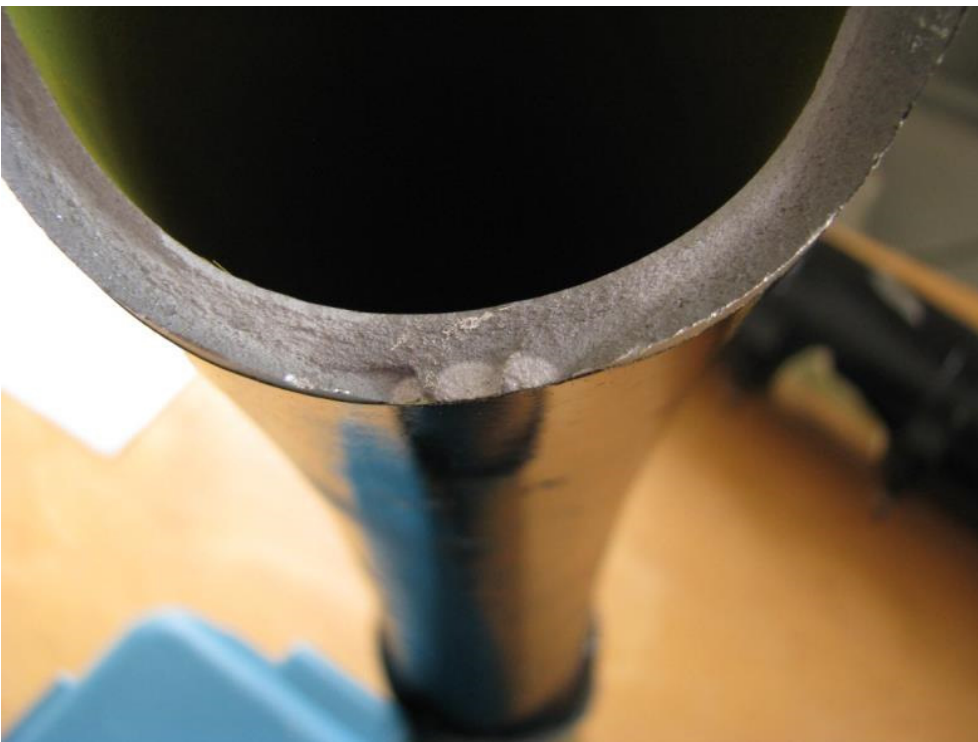
Image 4: Fracture surface of the smaller fracture piece including cracks
