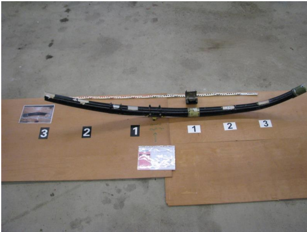
Image 8: Cross tube overview with the six examination areas
