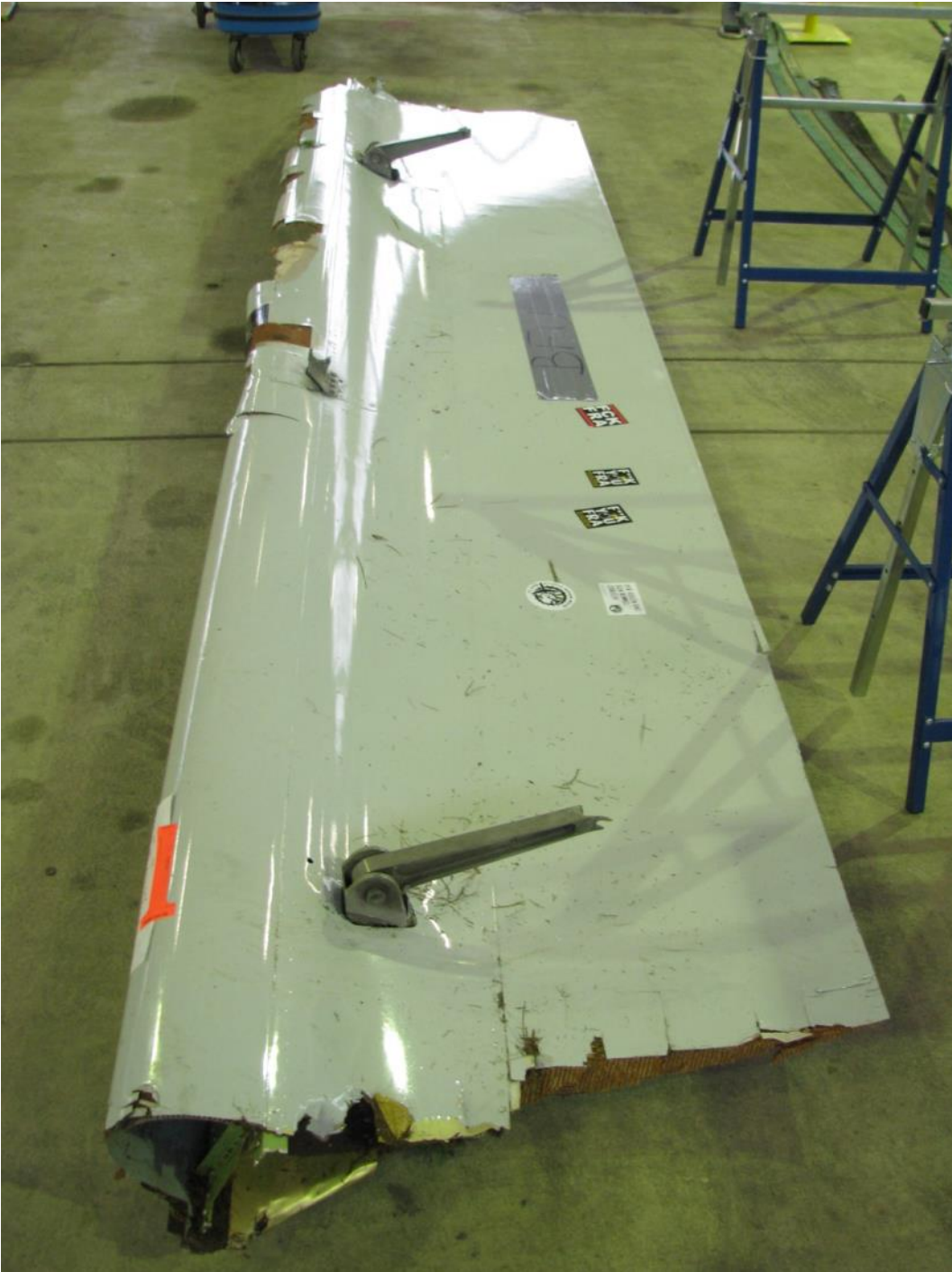
Image 4: Fractured flap part
