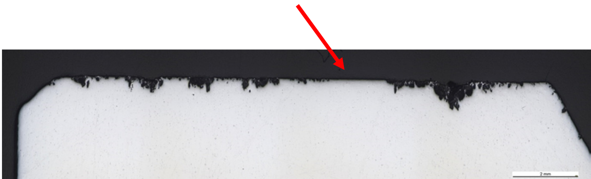
Image 17: Metallographic overview of the heavily corroded inside with lubrication groove (arrow)
