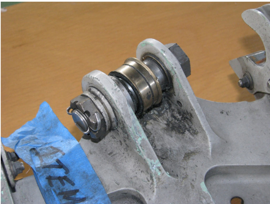
Image 9: Pin with bronze socket at the carriage
