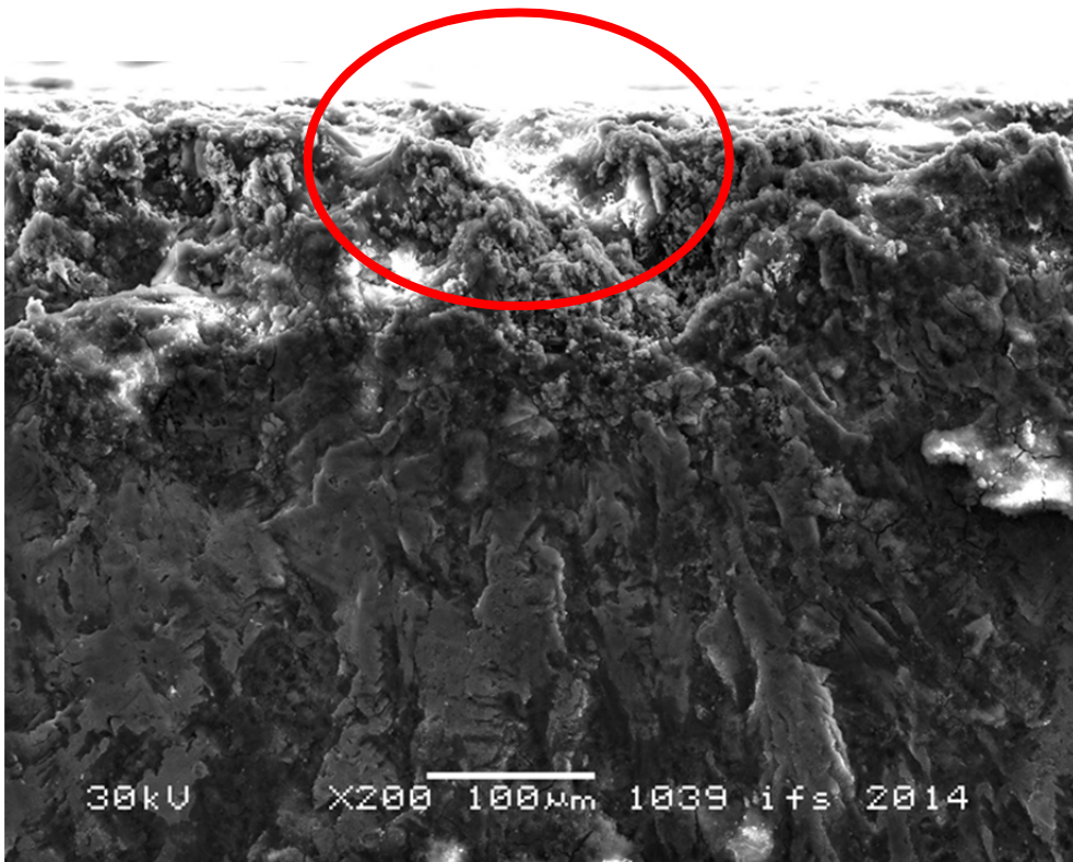
Image 13: Fracture origin with corrosion
