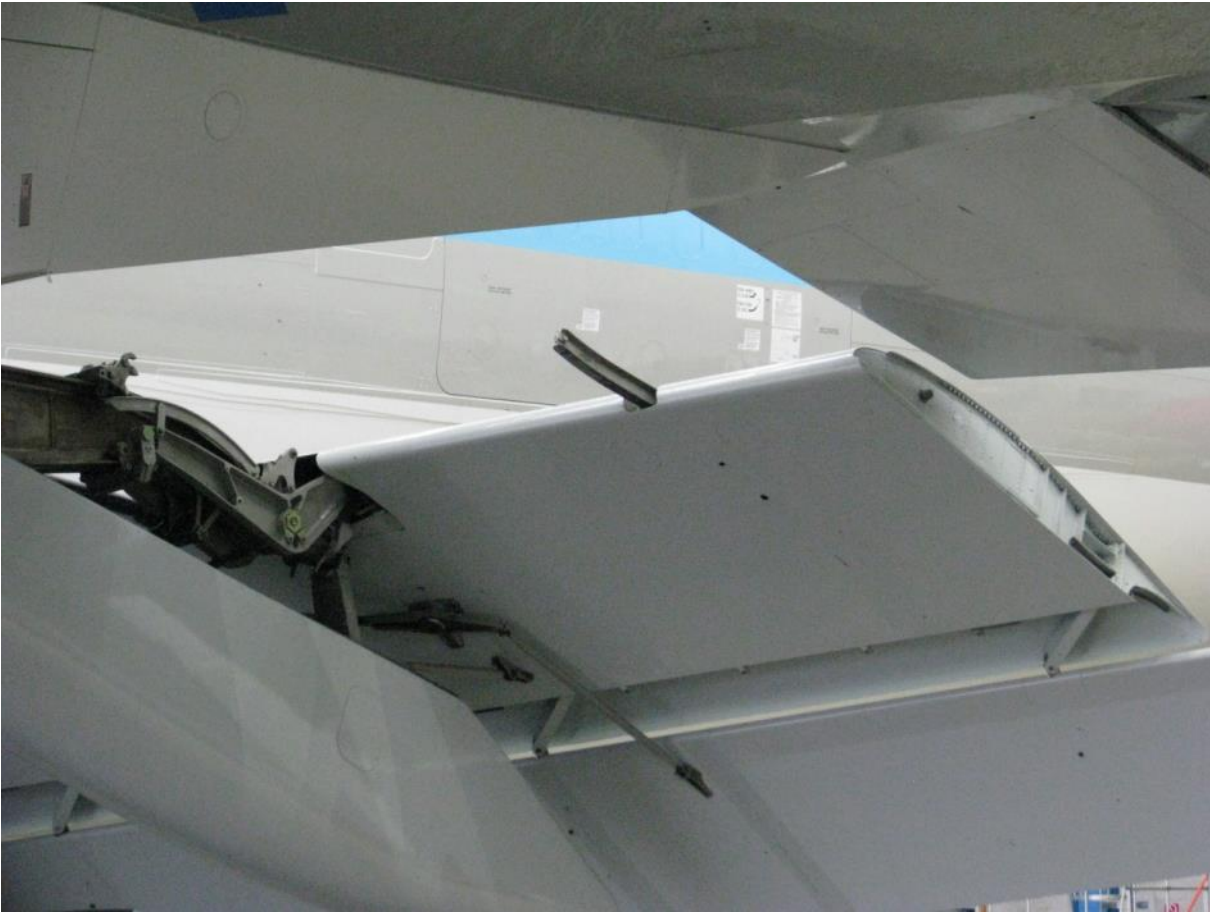
Image 1: The fractured flap viewed from below
