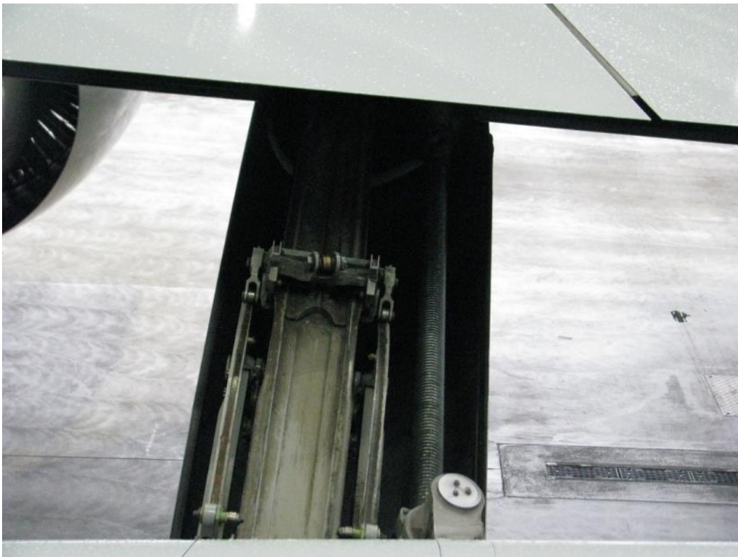
Image 3: Outer mounting point of the flap
