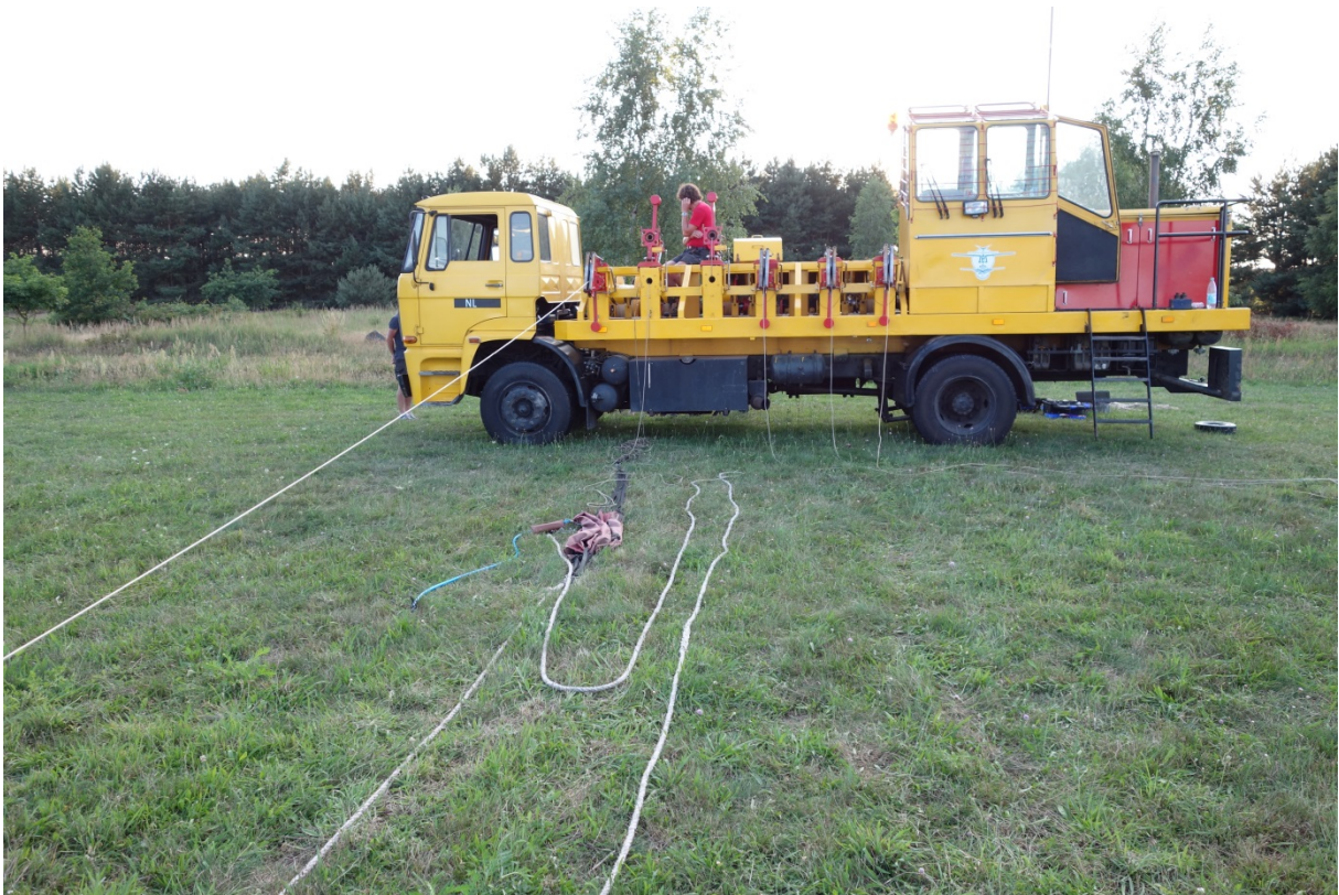
Six cable drum launch winch Busio
