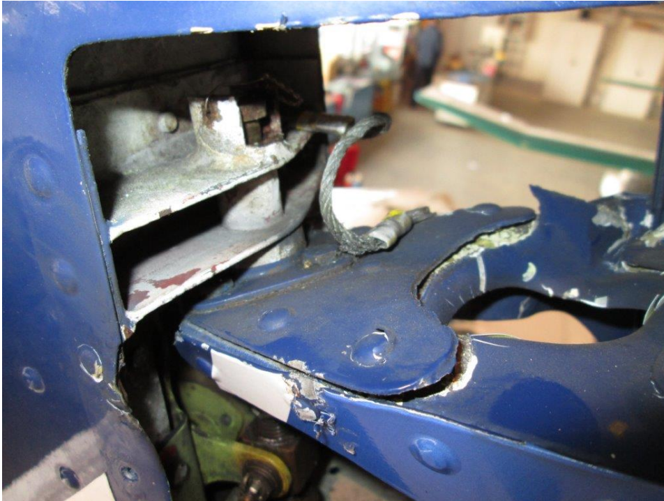
Image 3: Damaged centre rudder hinge
