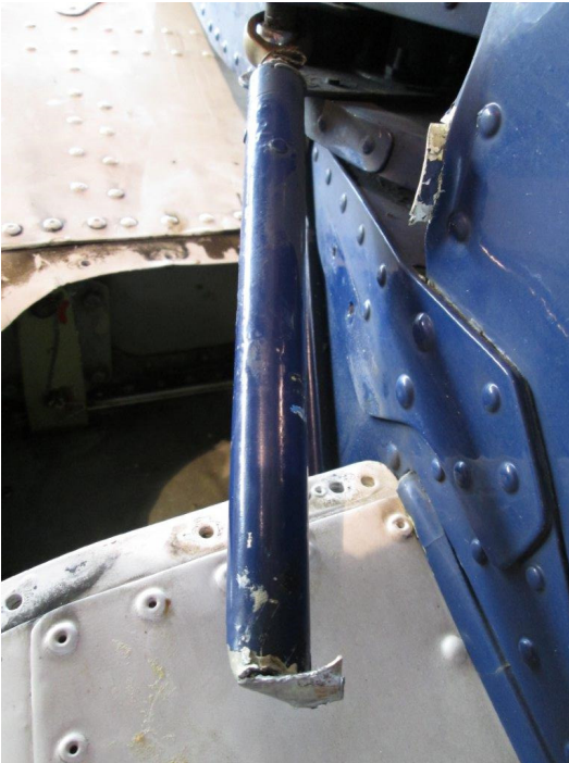
Image 2: Torn-out control rod
