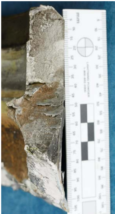
Figure 3: Discoloured and grey fracture zones
