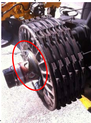
Figure 1: No. 4 axle with remnants of wheel hub (circled).
