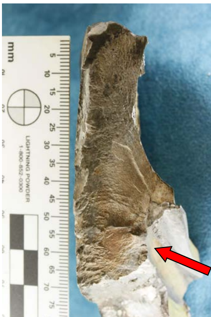
Figure 4: Fracture surface of the small piece; note the chevron origin at the bearing shoulder radius (arrowed).
