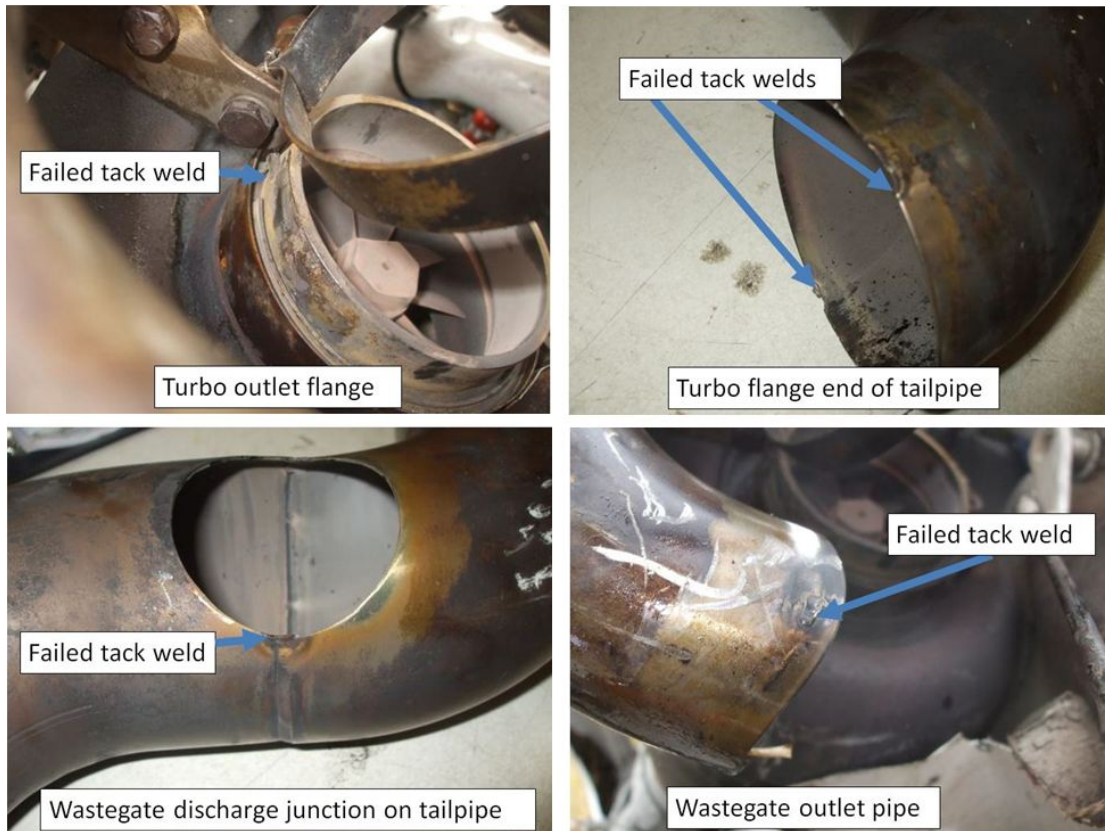
Figure 3: Failed tack welds
