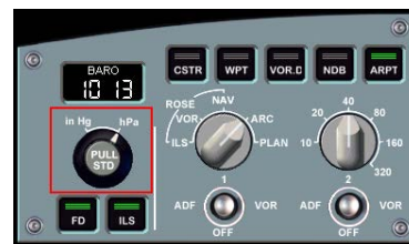
A320 EFIS control panel
