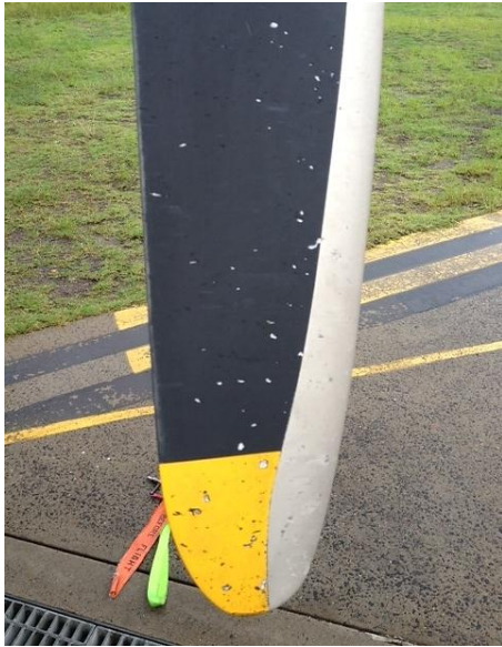
Figure 1: Propeller blade damage
