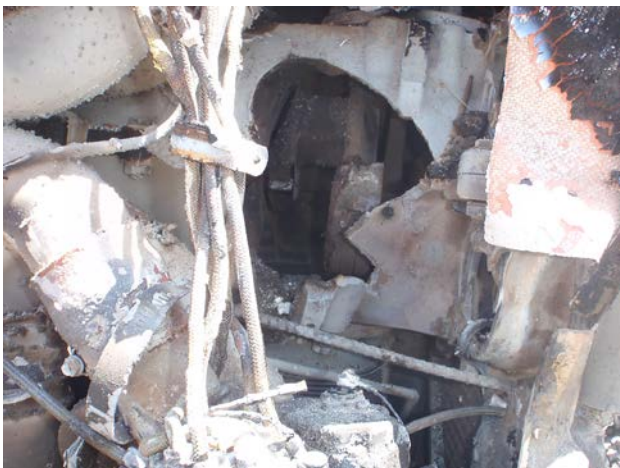
Figure 2: Engine damage to VH-HGZ
