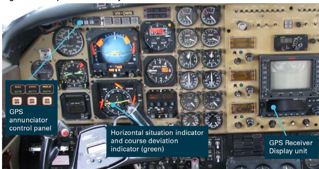
Figure 5: Cockpit instrument layout of VH-OWN
