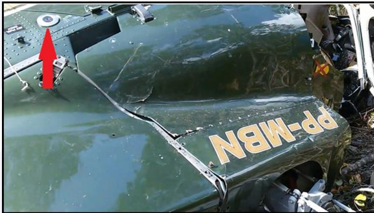
Figure 10 - Preserved Reservoir nozzle.
