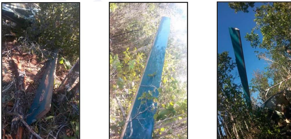
Figure 3 - Main rotor blades without impact on the leading edge.
