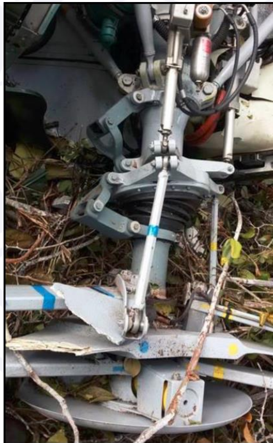
Figure 5 - Main rotor blade pitch control rod.
