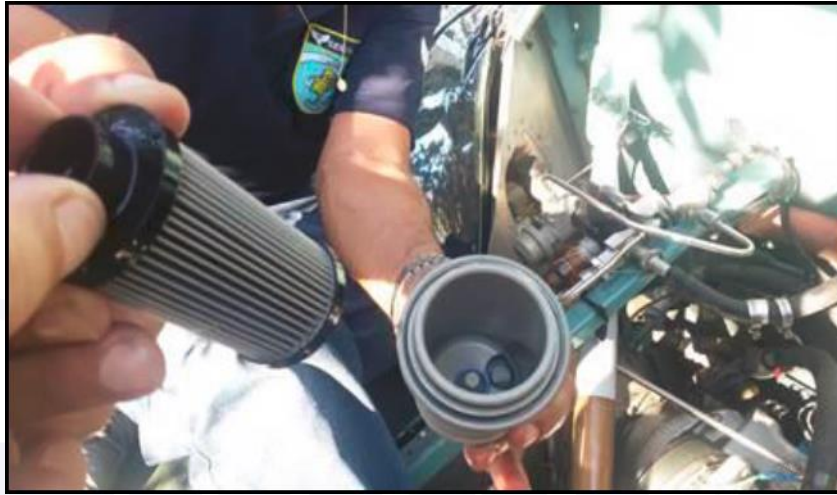
Figure 12 - View of the housing of the fuel filter element.
