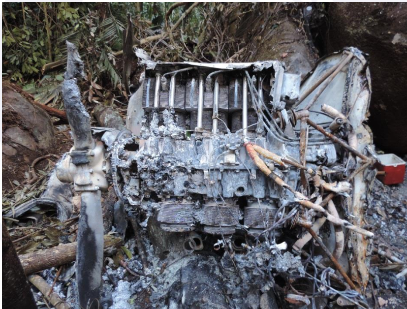
Figure 7 - View of the engine and propeller damaged by fire.
