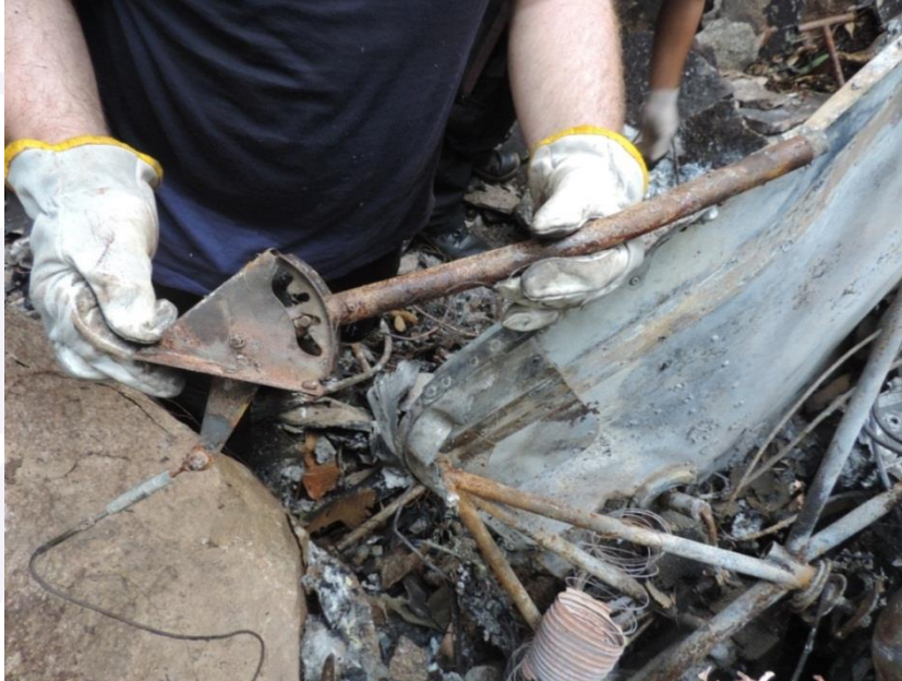
Figure 6 - View of the flaps control lever.
