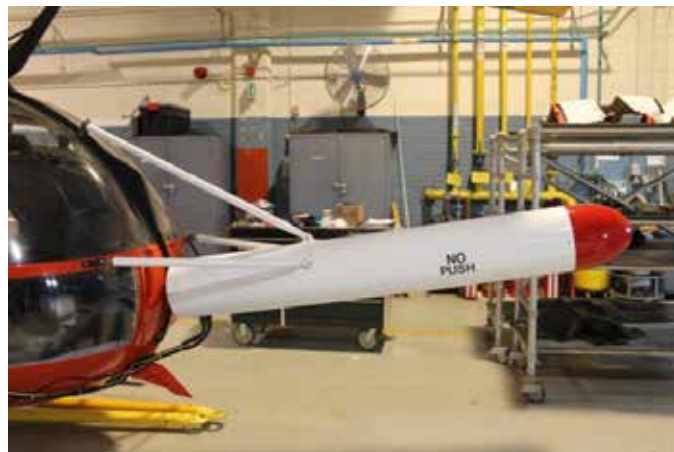
Photo 3. Ice probe attached to the nose of the helicopter
