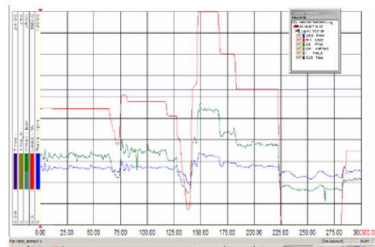
Graph 2: engine run 5 minutes before the power loss, nothing unusual noted by pilot, data shows fluctuations in the rail pressure
