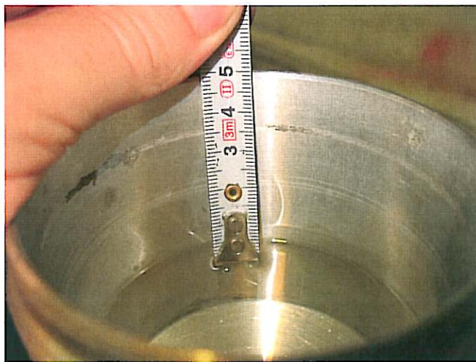
Picture 10 Fuel filter housings after removing the fuel filter
