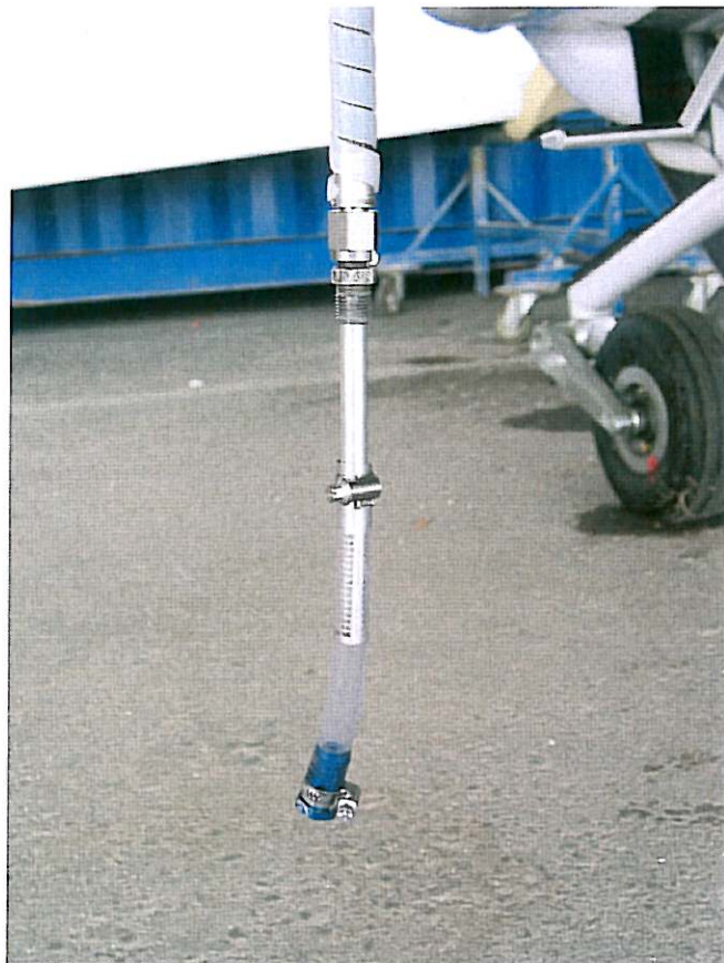
Picture 1 sealed finger filter of the main tank
