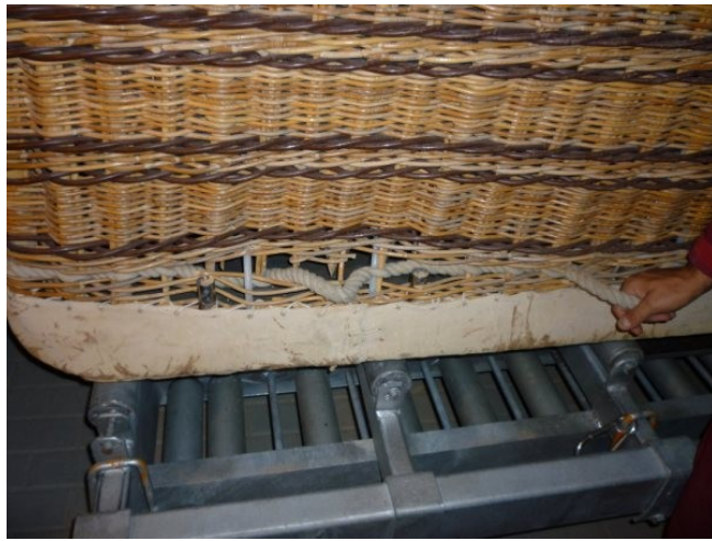
Balloon Basket Impact Damage
