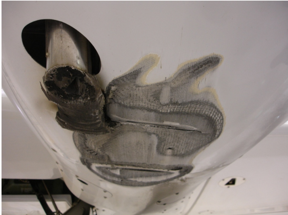
Figure A1-2 : Damaged Left Hand Exhaust Tube and Bottom Engine Cowling
