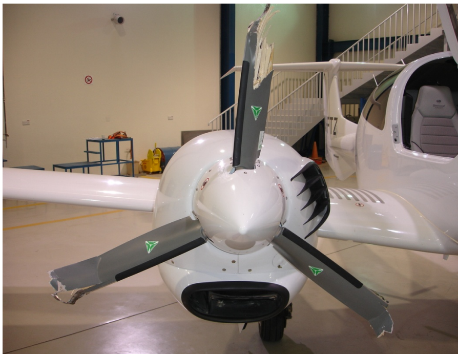
Figure A1-6 : Damaged Right Hand Propeller Blades
