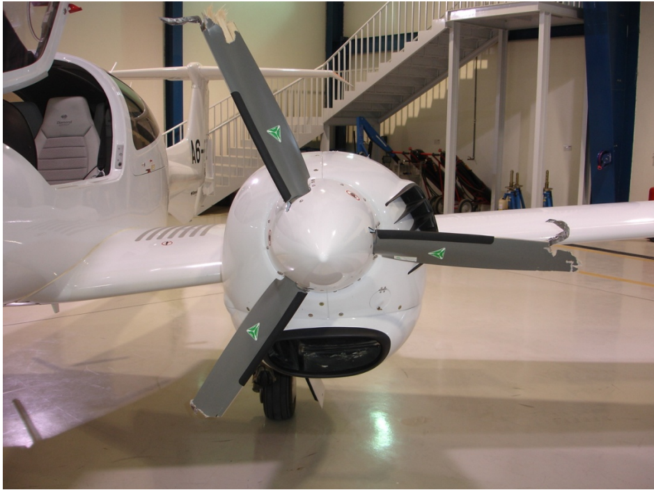
Figure A1-1 : Damaged Left Hand Engine Propeller Blades
