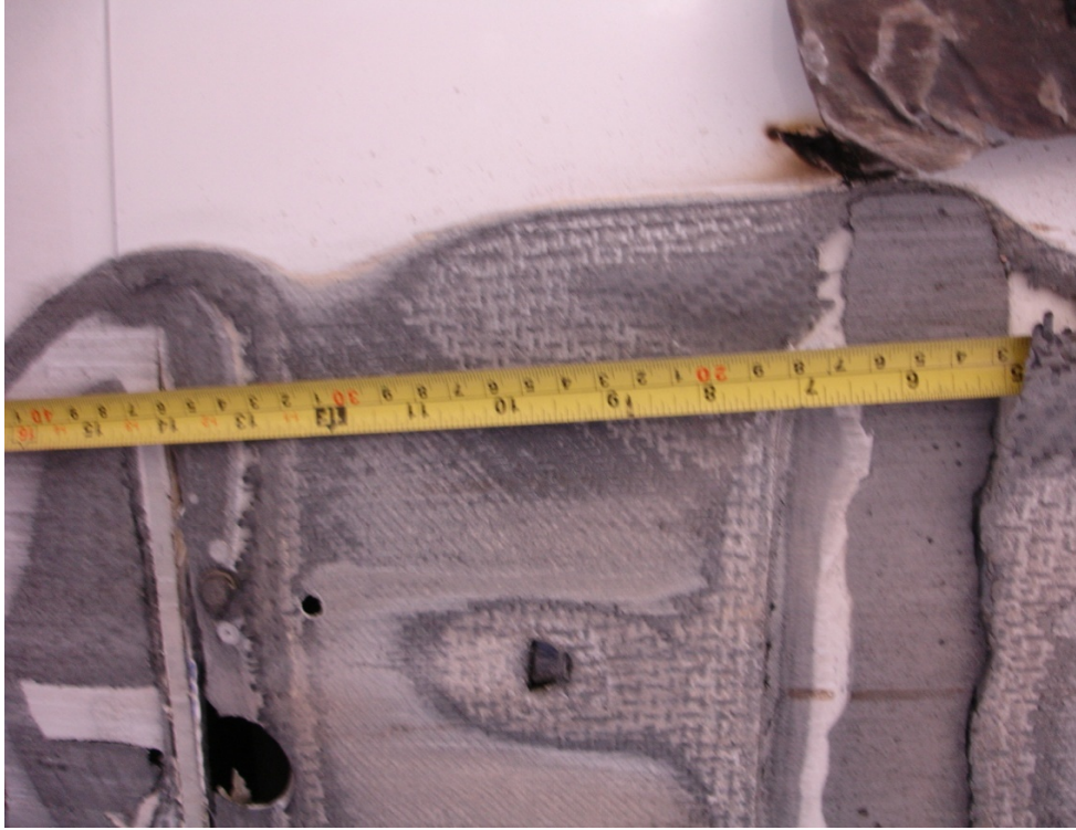
Figure A1-7 : Damaged Right Hand Exhaust Tube and Bottom Engine Cowling
