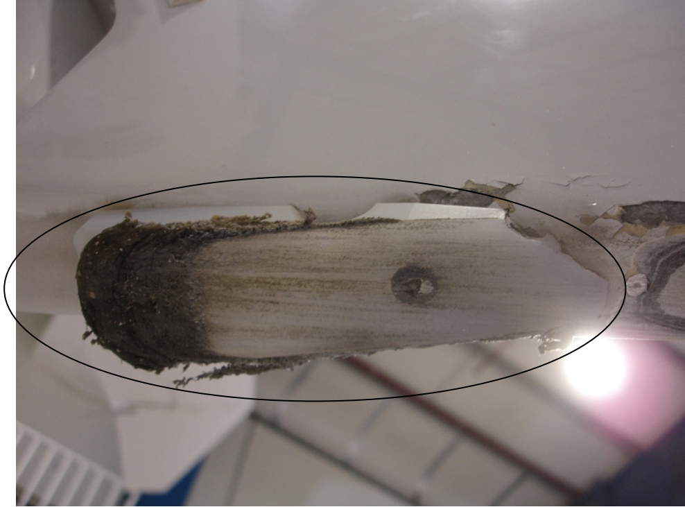
Figure A1-12 : Tail Skid Destruction
