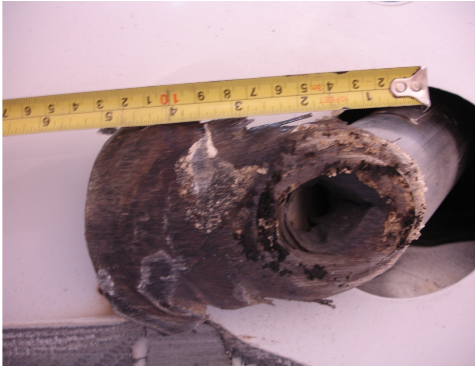
Figure A1-8a : Damaged Right Hand Exhaust Tube with a flat cut of 15 cm length
