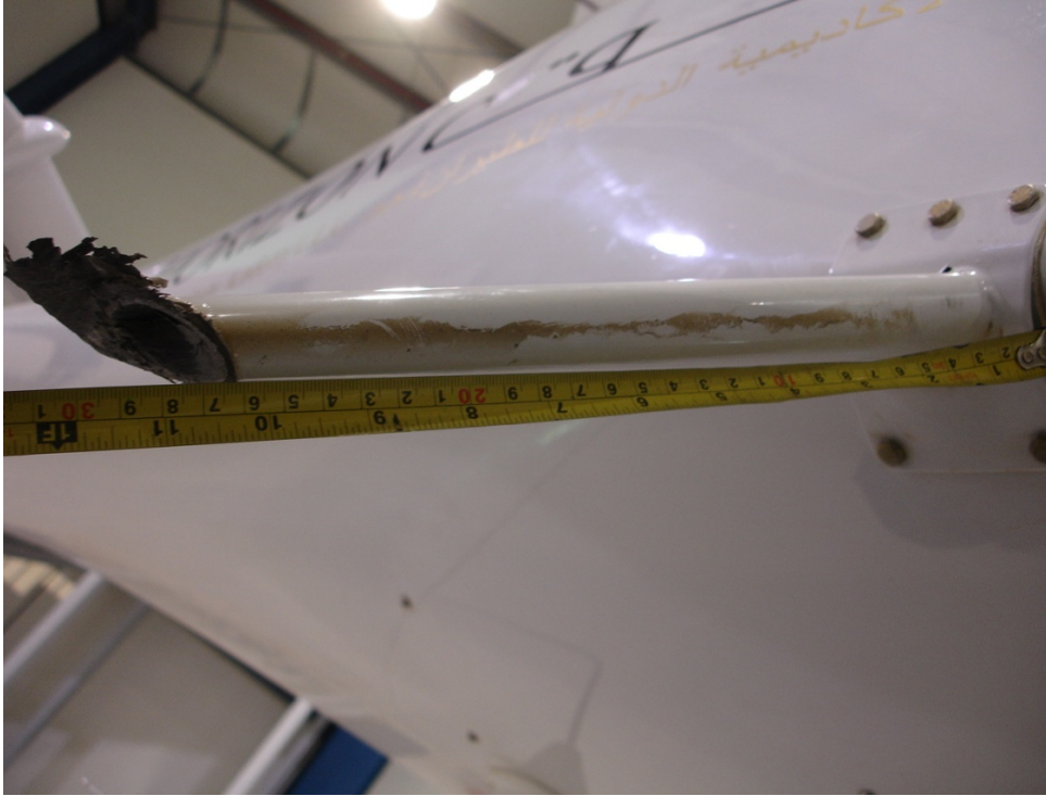
Figure A1-9 : Worn-out Damage Right Hand Foot Step
