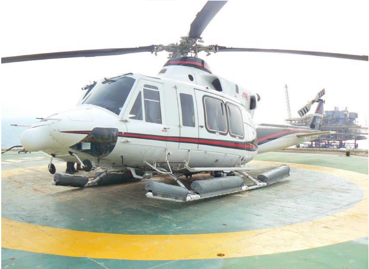
Photo 2. A6-FLZ following aft crosstube failure
