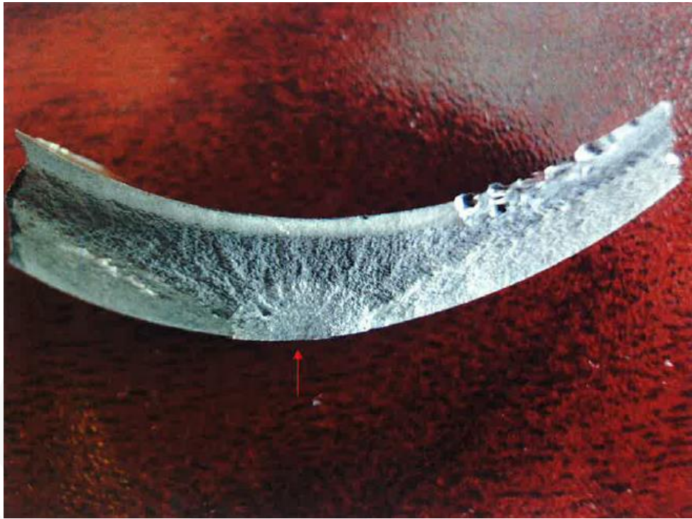
Photo 19. The fractured surface
