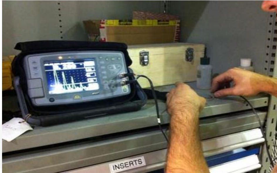
Photo 15. The ultrasonic equipment used to measure the failed crosstube.
