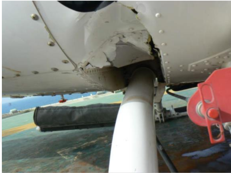
Photo 4. Damage to Fuselage Skin Panels and Aft Crosstube Tunnel Skin Panels.
