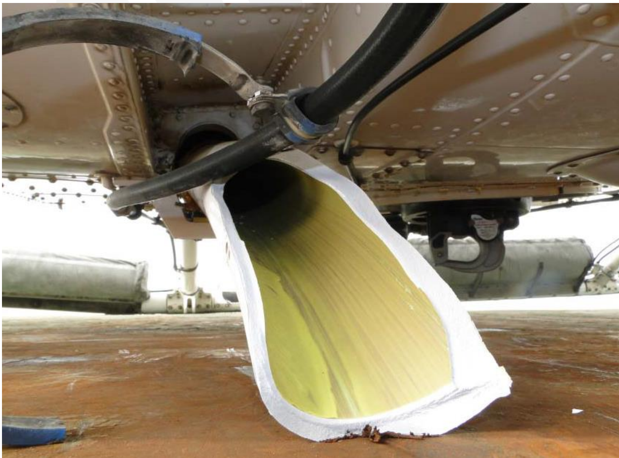
Photo 5. Fractured crosstube attached to the helicopter.
