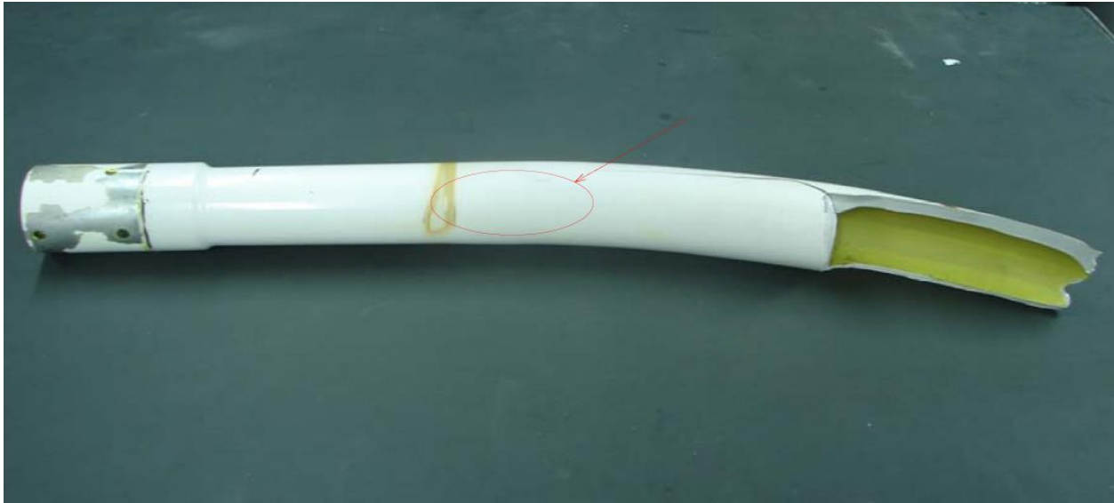
Photo 12. A6-FLZ failed crosstube as received in the metallurgical laboratory.
