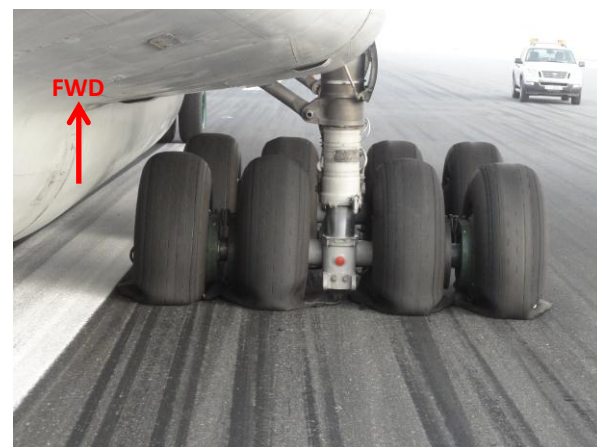
Figure 1- Skid marks at the runway
