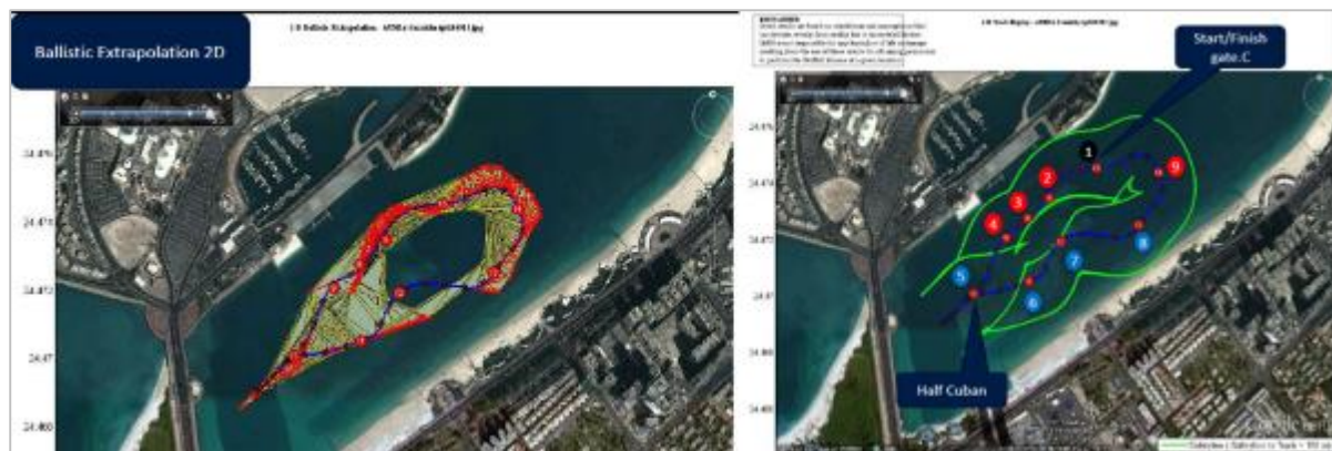
Figure8. Plan view of the trajectory analysis (left) and the Race Box safety line (right)
