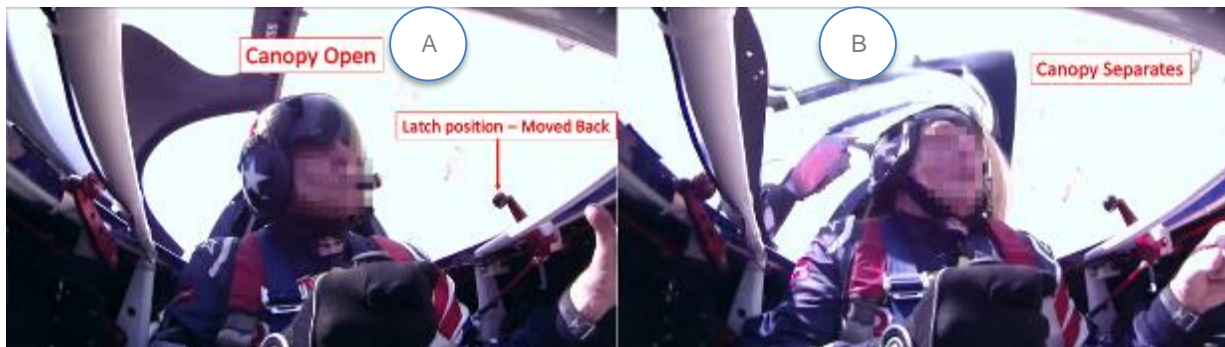
Figure 12. Photo showing canopy opening and separation (Source: on-board camera)
