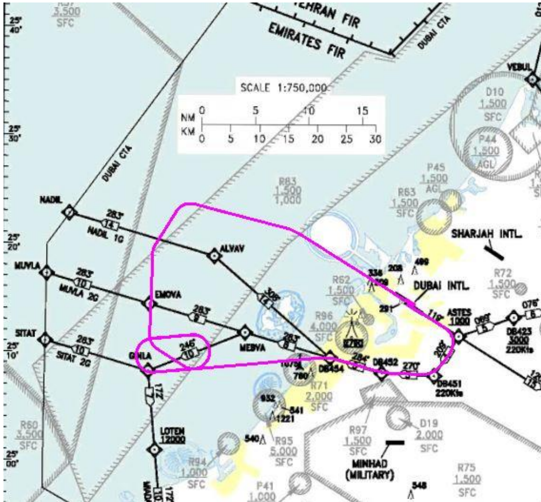
Figure 1. Flight path on RNAV 1 3 SID runway 12R chart
