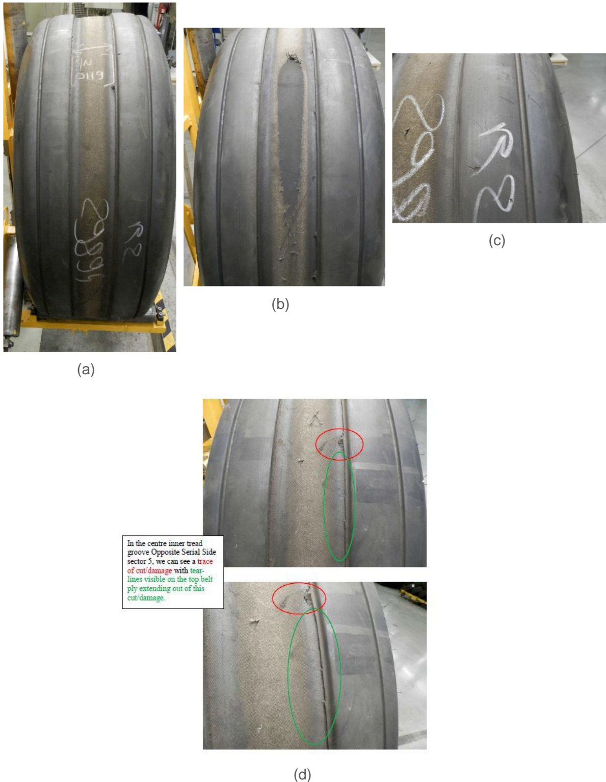
Figure 16. Damaged tire [Source: Michelin]
