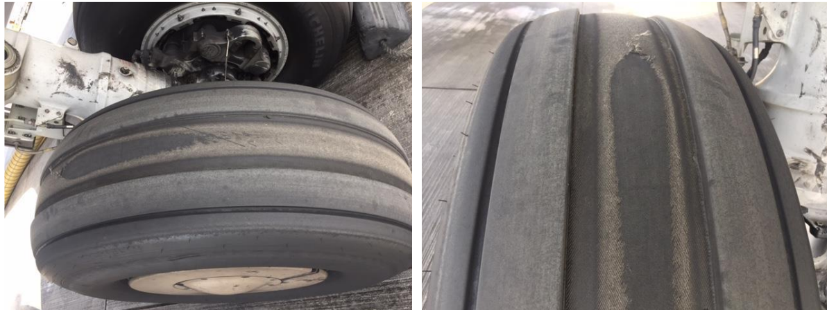
Figure 4. Damaged No. 1 tire (left outboard tire)
