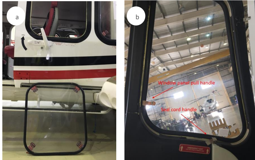
Figure 9. Aircraft cabin escape window and example of left flight deck escape window
