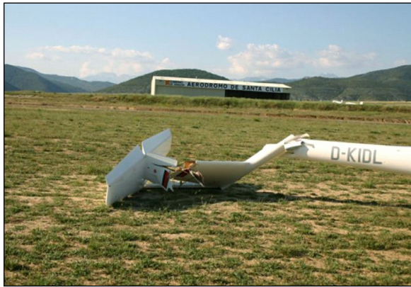
Figure 1. Damage to aircraft D-KIDL
