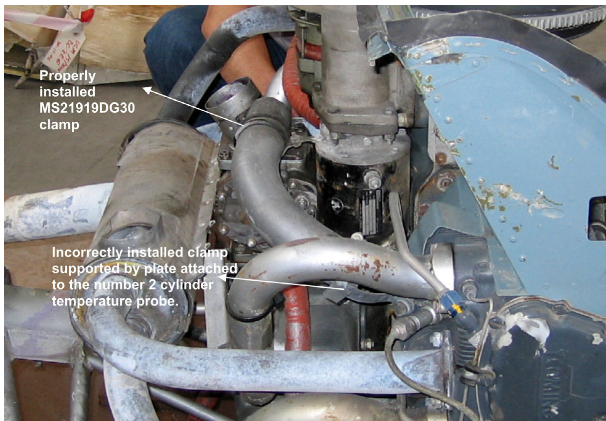
Figure 3. Alternative air tube installation
