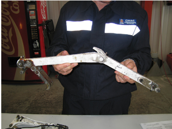
Figure 5. Condition of the lower side link following the accident
