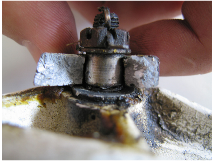
Figure 3. Break of the bellcrank lug
