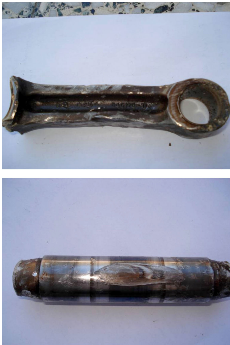
Figure 4. Connecting rod and pin found along the landing run
