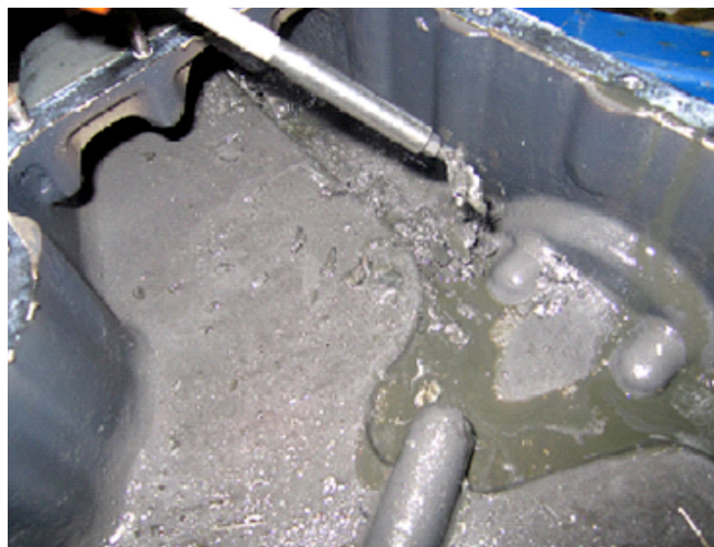
Figure 4. Metal particles and shavings in the crankcase
