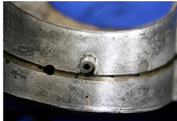
Figures 4 & 5. Deformations in the central half bearing and half casing
