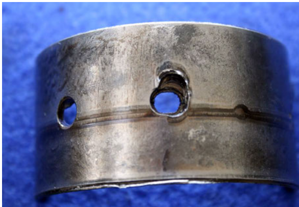
Figures 4 & 5. Deformations in the central half bearing and half casing
