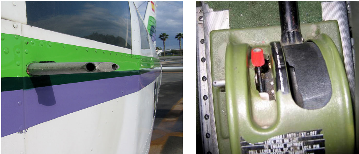
Figure 4. View of the pitot/static tube that supplies information to the BGE. Emergency gear lever
