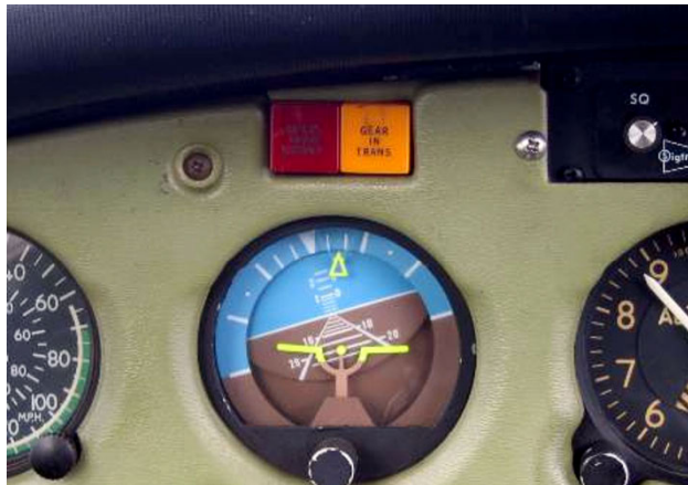
Figure 3. Photo of the gear in transit lights (yellow) and gear unsafe light (red)
