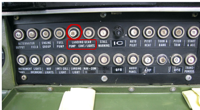
Figure 6. Close-up of the position of the landing gear pump breaker
