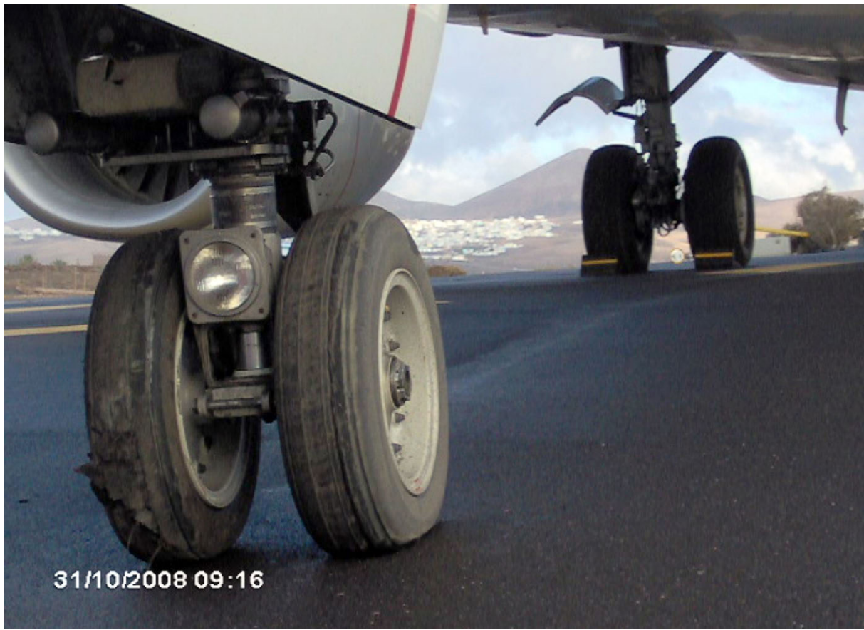
Figure 2. Damage to the nosewheel landing gear
