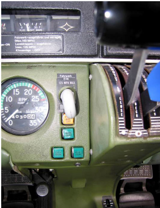
Figure 2. Photo of gear lever and associated lights
