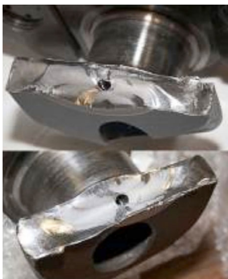
Figure 9. Fracture in the crankshaft
