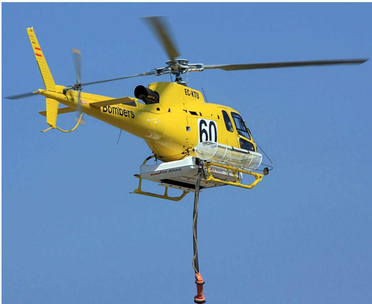
Figure 1. Helicopter with the Simplex 310 firefighting system attached
