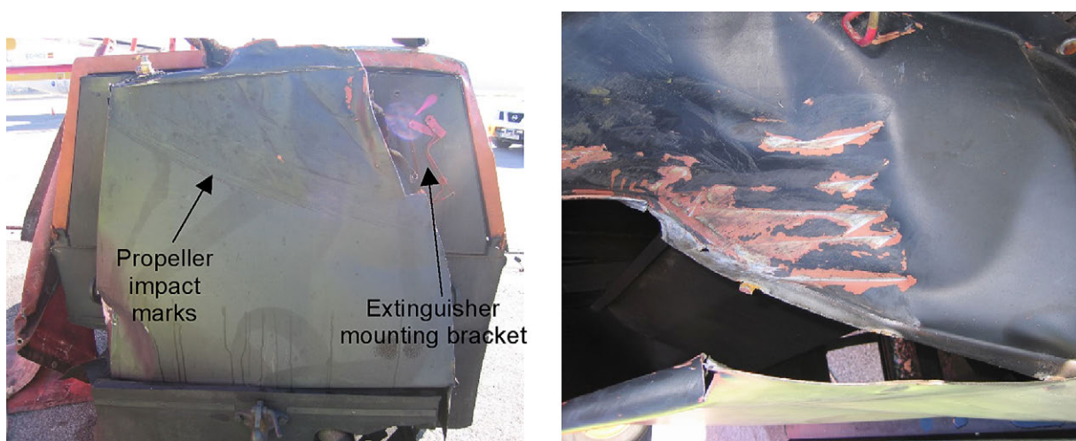
Figure 2. Photographs of the GPU. Left: impact marks on the rear of the unit. Right: Close-up of the impact marks
