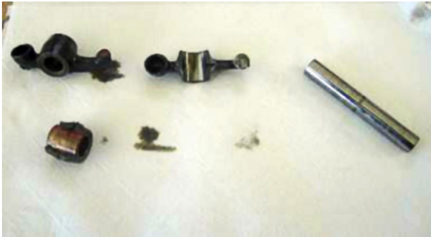
Figure 6. Rocker arms and axle from the no. 2 cylinder
