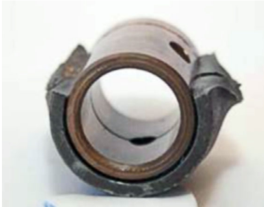
Figure 8. Misalignment of the lubrication orifices
