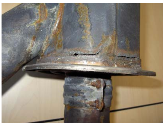
Some cracks in the exhaust muffler
