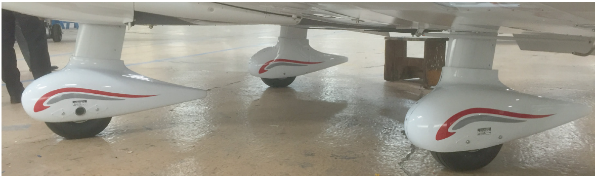
Figure 3: DR400 landing gear strut and wheel fairings. (Photo: Dutch Safety Board)
