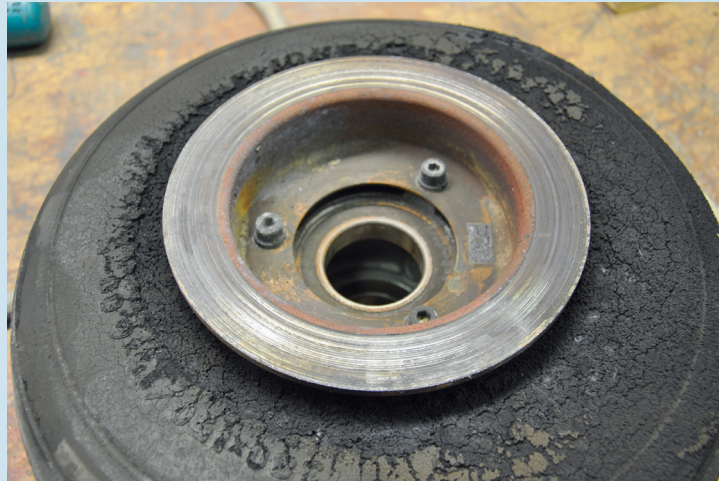
Figure 9: PH-HLR left wheel with damaged tyre and brake disc. (Photo: Dutch Safety Board)
