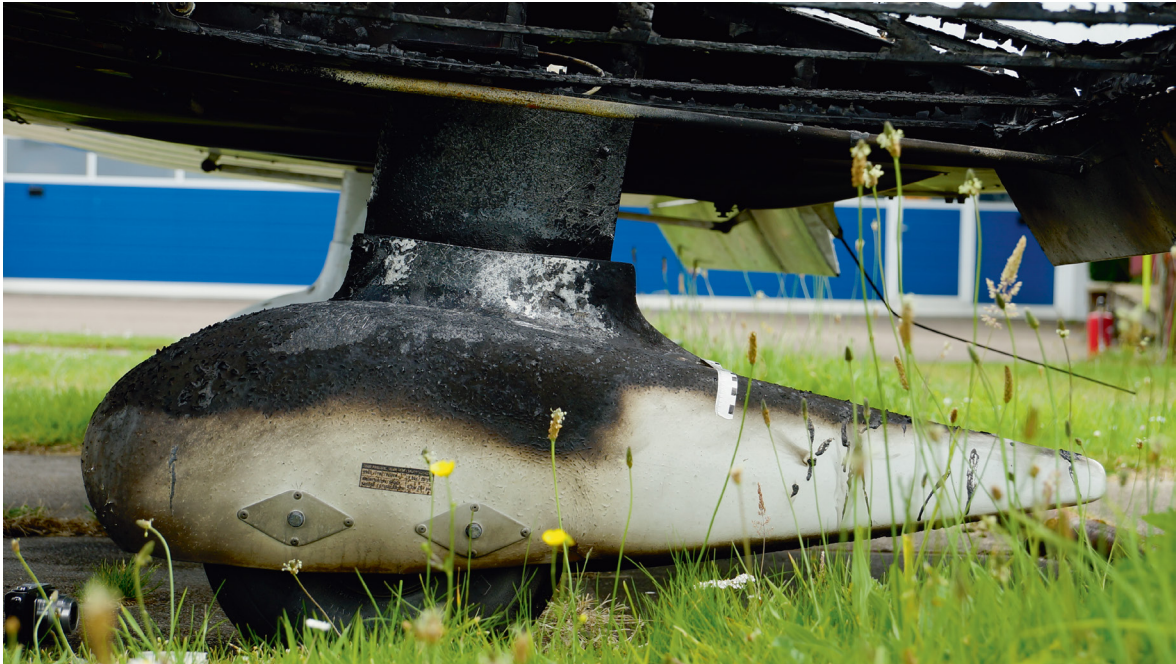
Figure 8: PH-HLR side view of left-hand wheel fairing and gear strut fairing, damaged by heat. (Photo: Dutch Safety Board)
