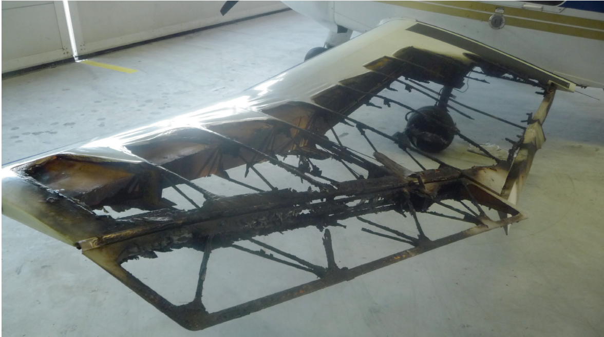
Figure 6: The PH-SPZ left-hand wing damage. (Photo: Dutch Safety Board)
