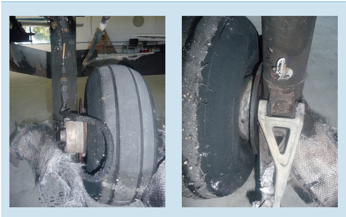
Figure 7: The destroyed left-hand main gear and strut fairing from PH-SPZ, seen from front (left picture) and from aft (right picture). (Photos: Dutch Safety Board)
