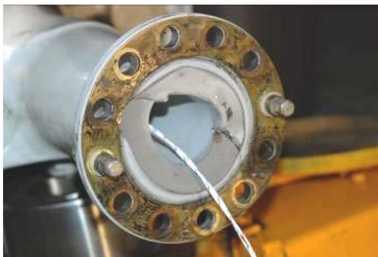
Figure 2: The fractured number-one axle showing that the failure occurred near the brake attachment flange
