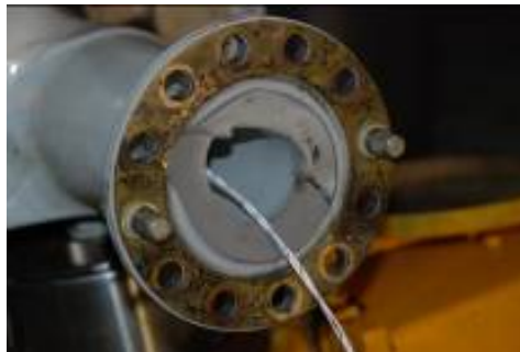
Figure 1: Broken axle. Failure occurred near the brake attachment flange
