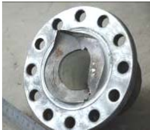
Figure 3: View of the fracture surface. The fatigue crack initiated from the 5 o'clock attachment hole
