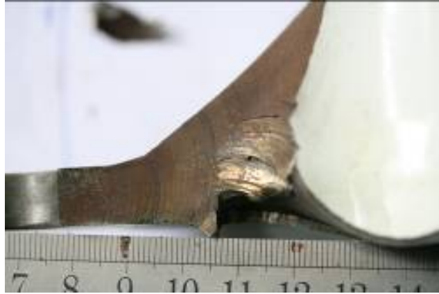
Figure 3: Beach marks started from the hole, propagated inward toward the axle.
