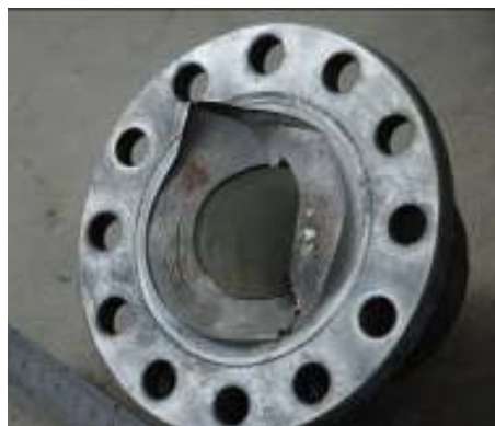
Figure 2: Fracture surface: final failure. Fatigue crack was initiated from the 5 o'clock attachment hole.
