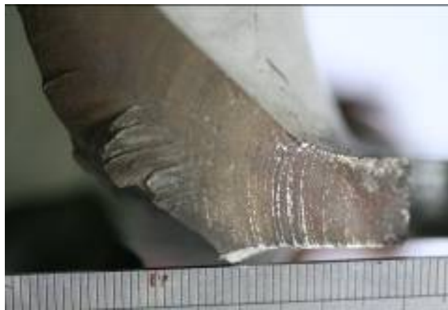
Figure 4: The appearance of fracture surface on the matching piece. Beach-marks reached approximately 8 cm from the hole.
