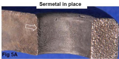
Figure 5A: Bore surface at fracture origin (arrow) with Sermetel coating in place.
