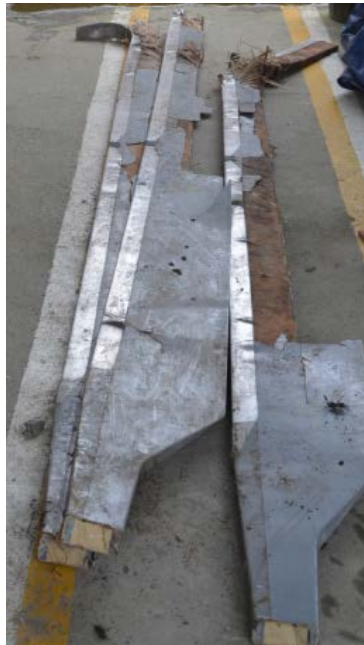
Figure 6: General condition of the Main Rotor Blades
