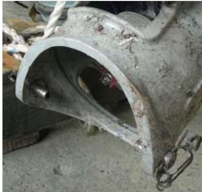
Connecting casing junction with missing Gimbal ring
