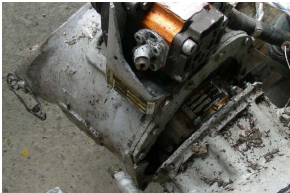
Connecting casing junction with MGB failure
