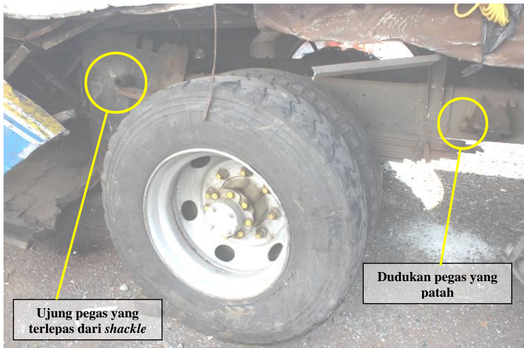
Gambar 12. Suspensi roda kanan-belakang Mobil Bus AD-1543-CF
